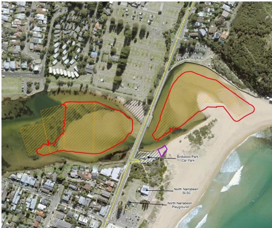
Figure 5-2: Area of excavation for 2021 entrance clearance campaign (Cardno, 2021)
