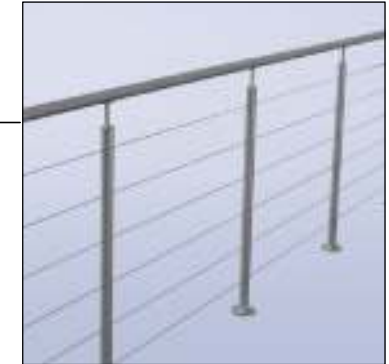
Marine grade stainless tubing & steel wire to perimeter of roof terraces
