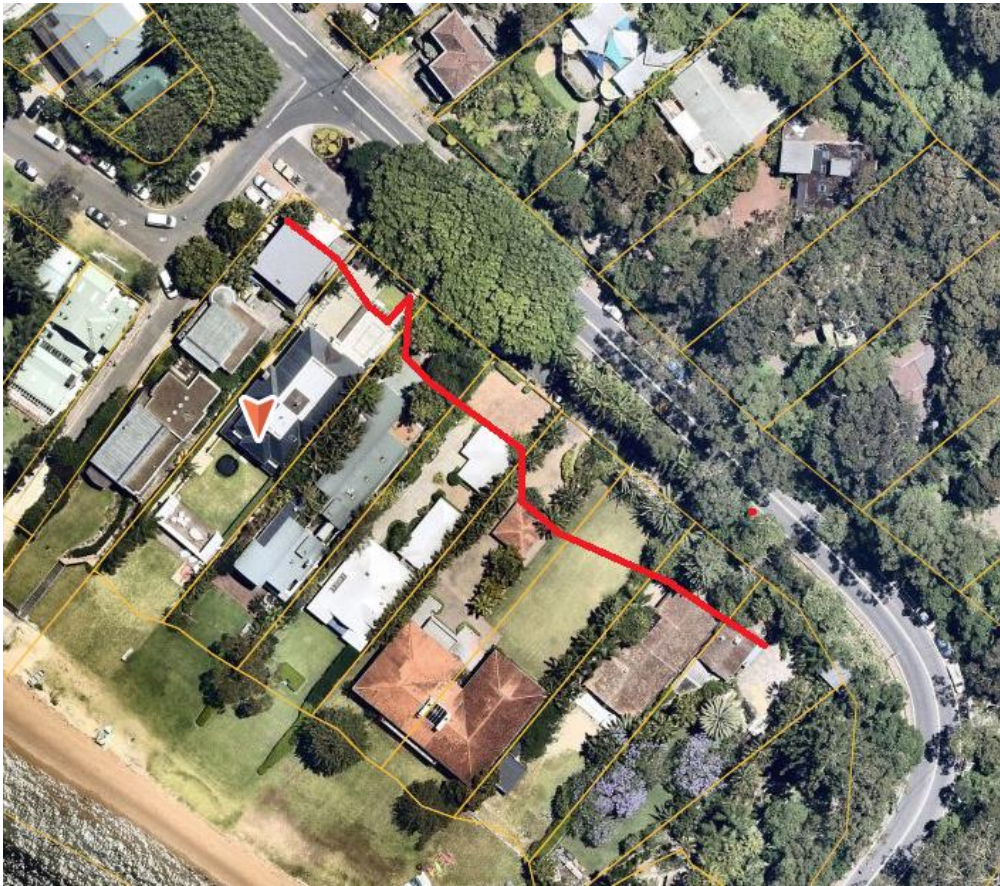
Figure 12 Established building line showed in red.
