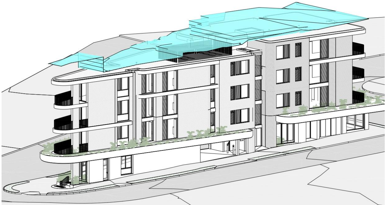
Figure 13: Building height blanket diagram showing compliance with the 14.3/ 16.9 metre building height standard
