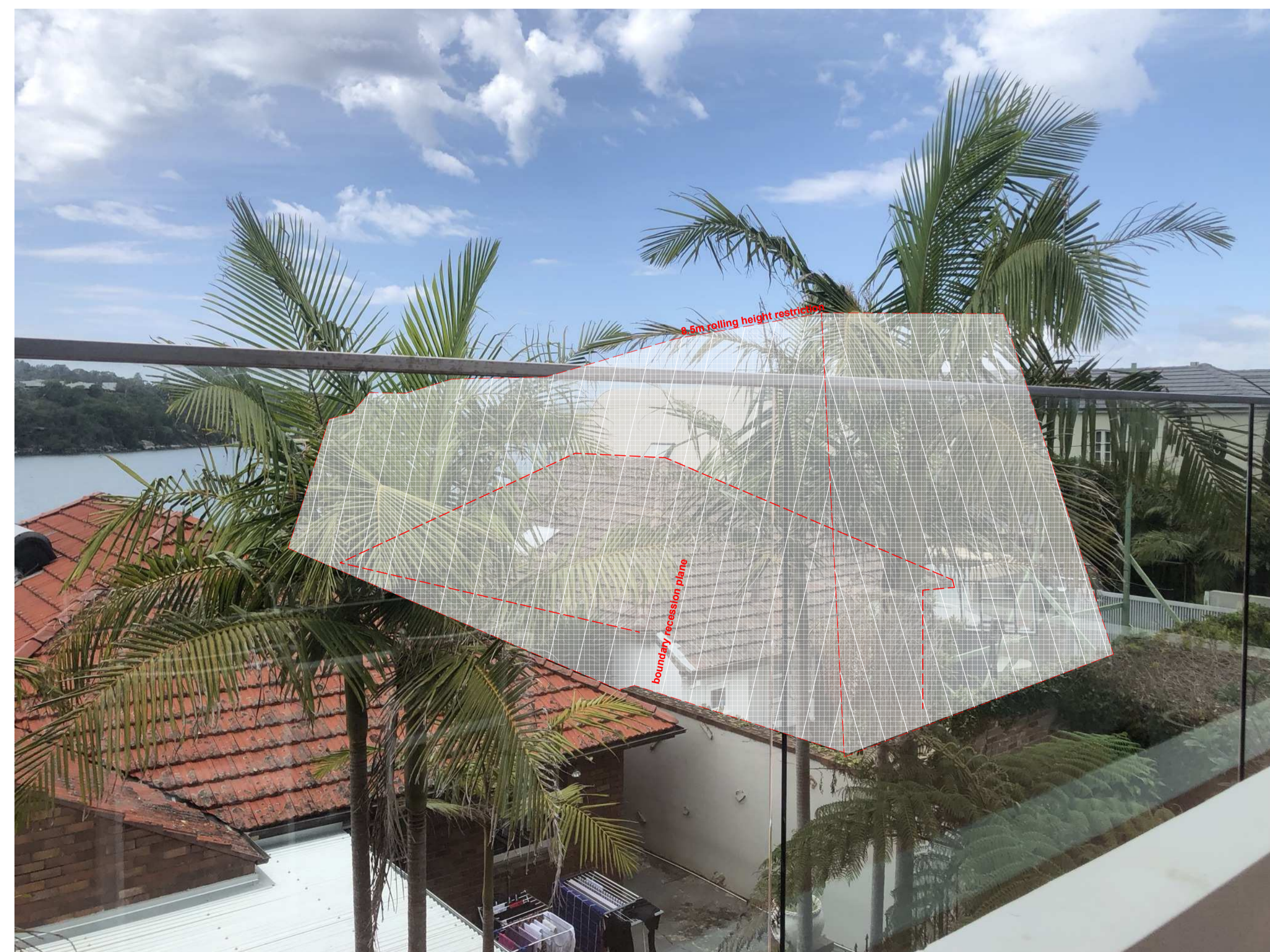
IMG_3580 6/22-26 Addison Road - Upstairs Living Room [PERMISSABLE] Daylight Recession Planes & 8.5m Rolling Height Plane Overlaid
