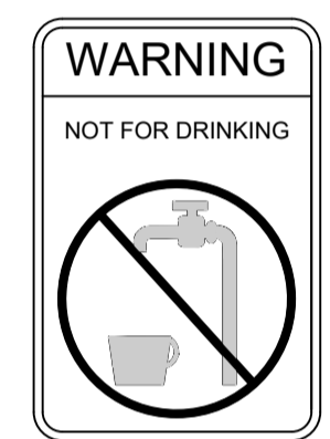
NON-POTABLE WARNING SIGN
