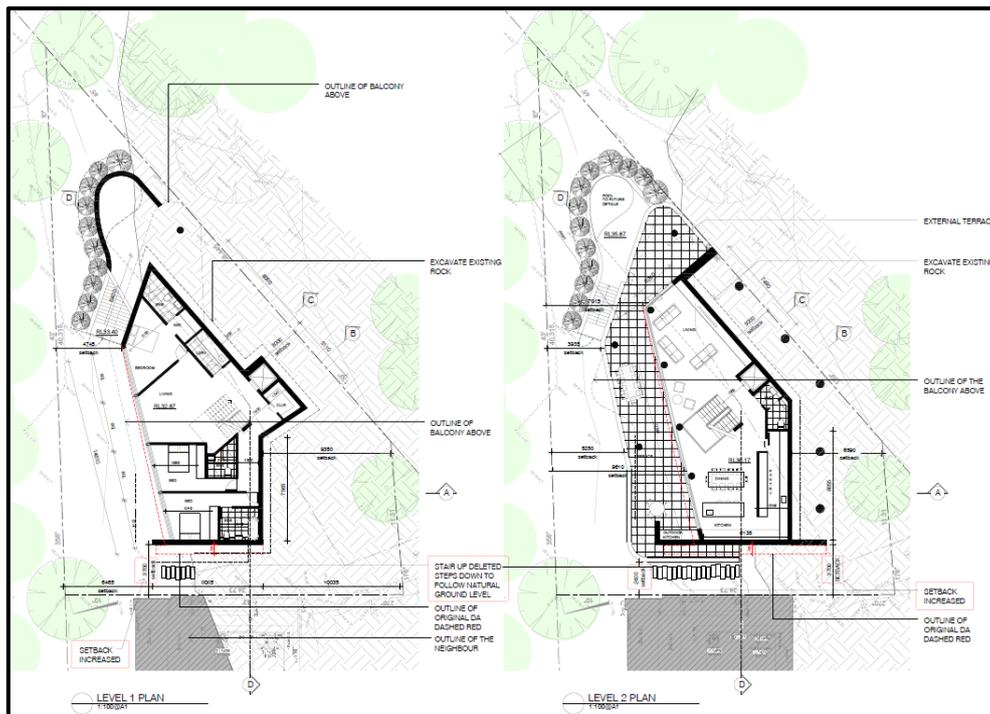
Figure 7: Excerpt of Level 1 and 2 plans noting the deletion of the southern stair access associated with the adjacent access driveway area to the east of the subject site
