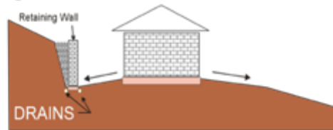
Fig. 5 Well Drained Sites
