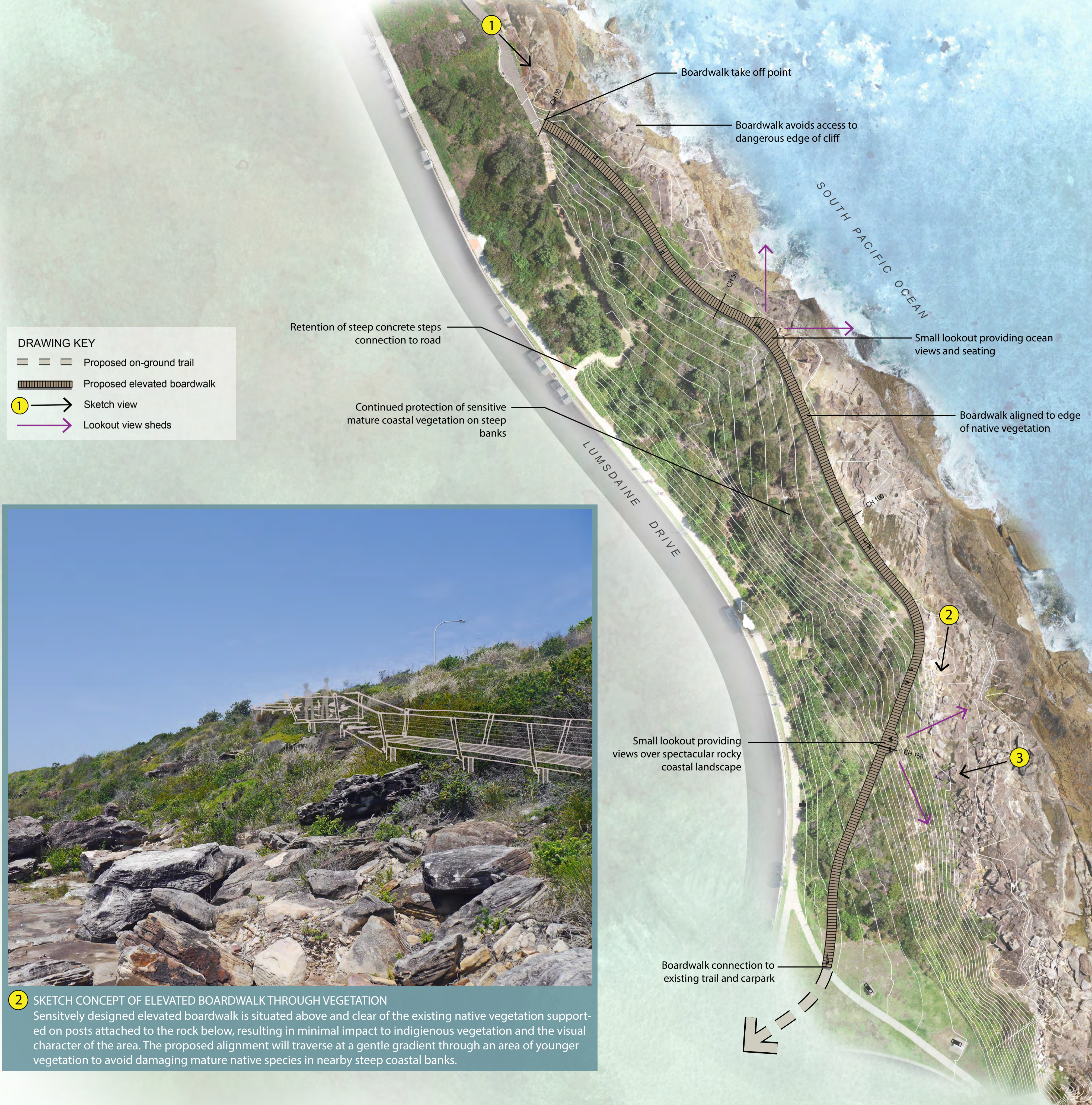
1 SKETCH CONCEPT OF BOARDWALK ENTRY The proposed elevated boardwalk diverges from the existing Curl Curl boardwalk and follows an existing desire line through low shrub vegetation. The boardwalk alignment is designed to provide visitors with a coastal experience that is safely set back from the cliff edge. Consideration of similar timber decking materials to match existing boardwalk or use FRP charcoal mini mesh for increased durability and grip.
