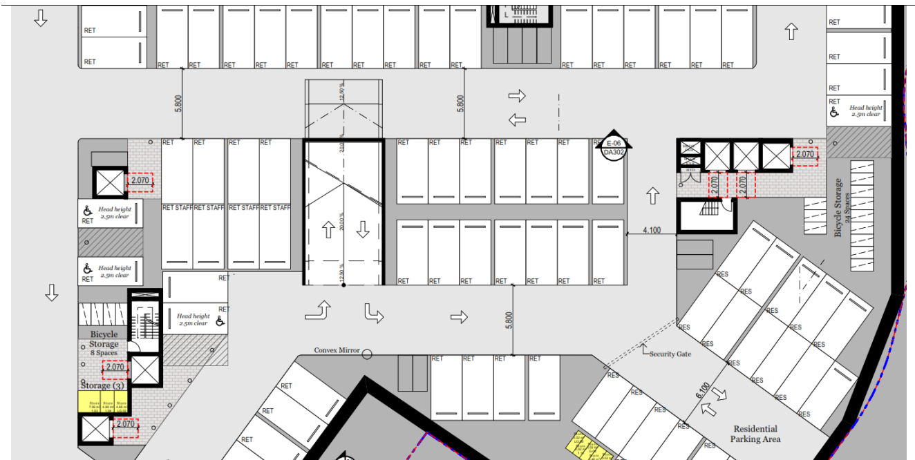
Basement 4 showing 4 accessible parking spaces allocated for Retail use.
