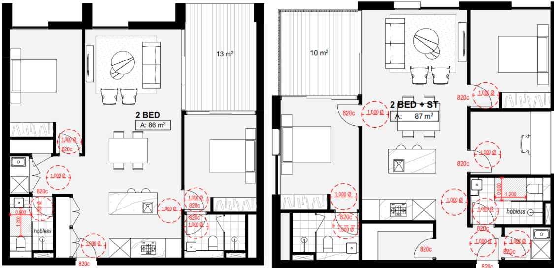
2 BED SILVER STANDARD LIVABLE HOUSING UNIT TYPE A Unit No. LG.03, LG.04, G.03, G.04, 1.03, 1.04
