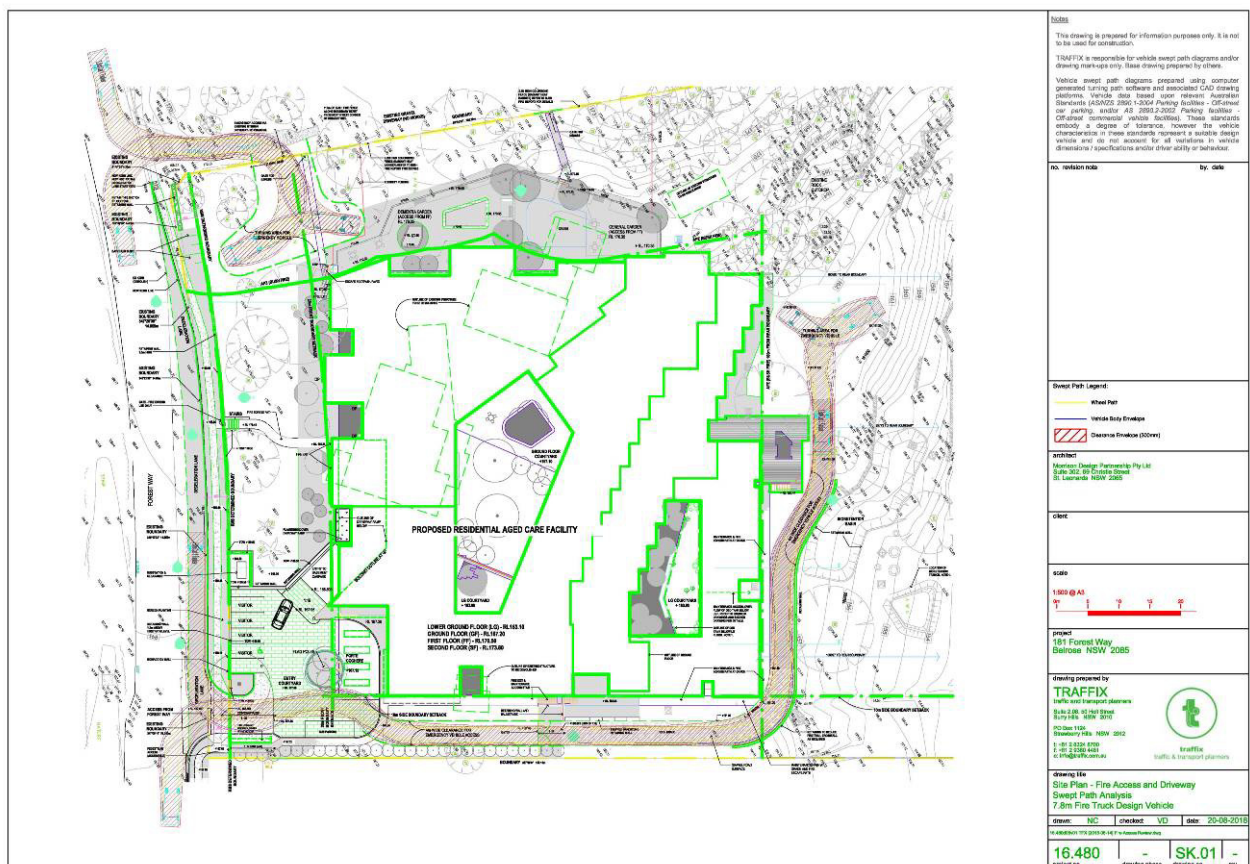
Figure 3.2 – Fire trail (swept path analysis)
