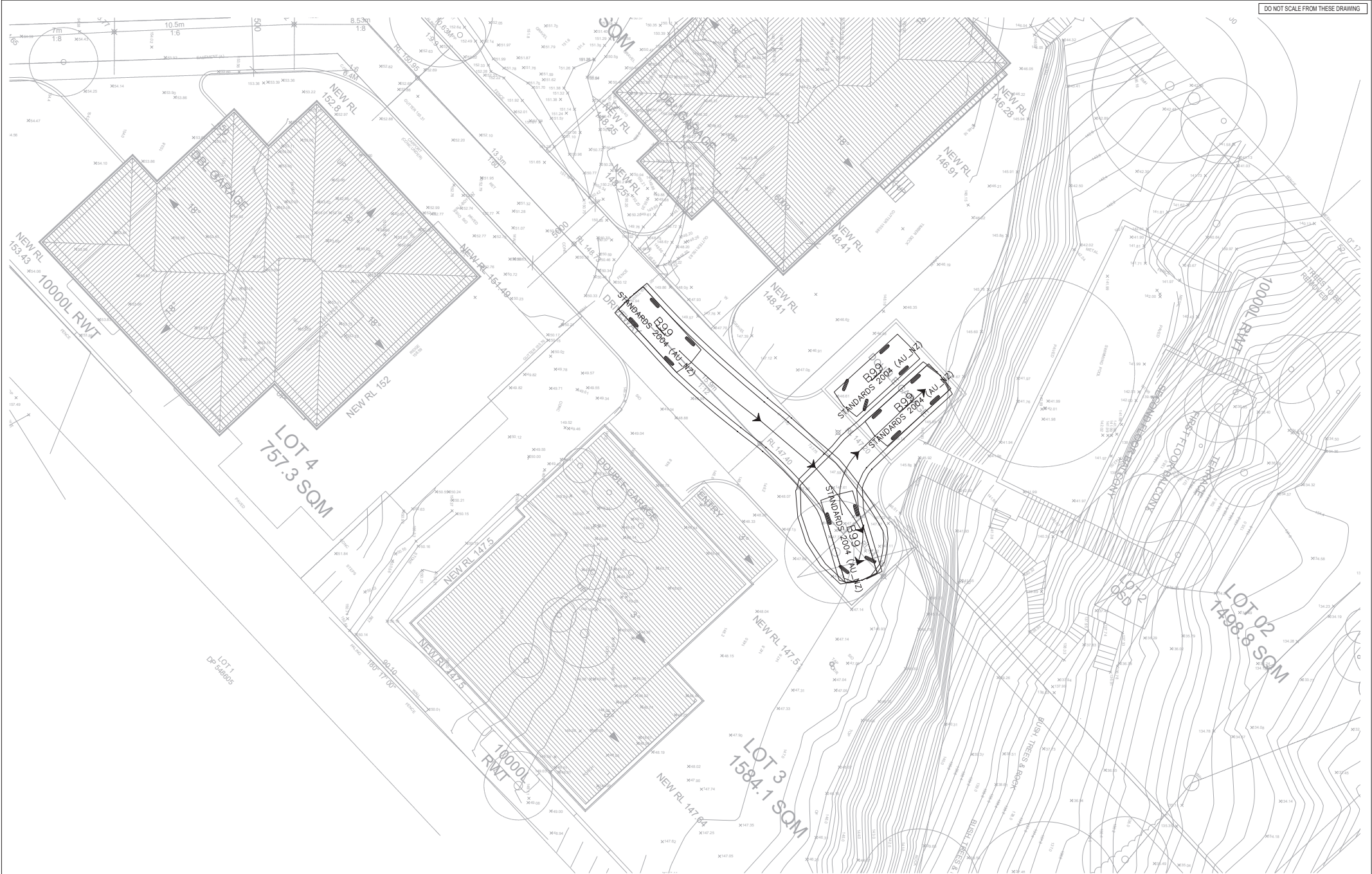
TURNING PATH ANALYSIS FOR B99 SCALE 1:100
