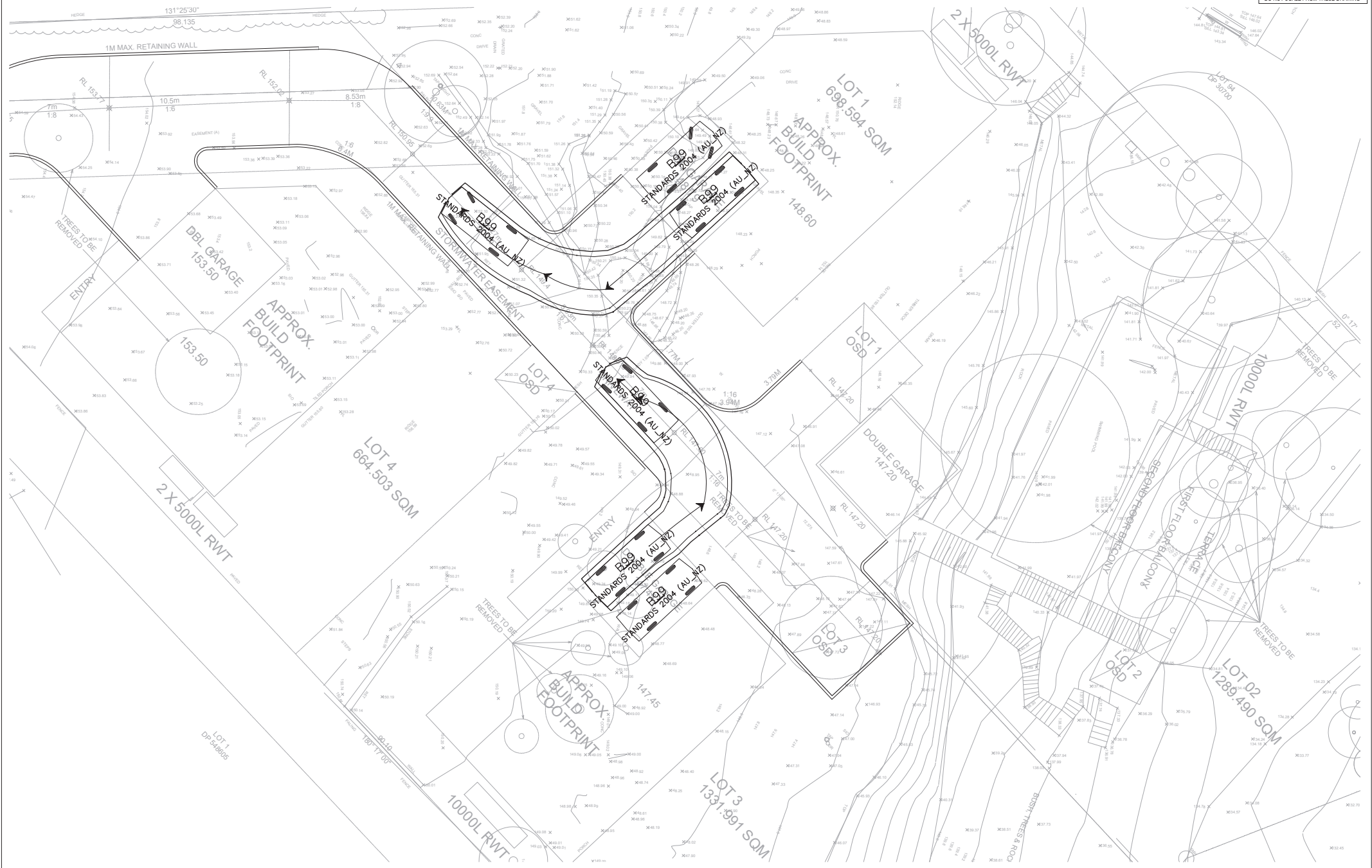
TURNING PATH ANALYSIS FOR B99 SCALE 1:100
