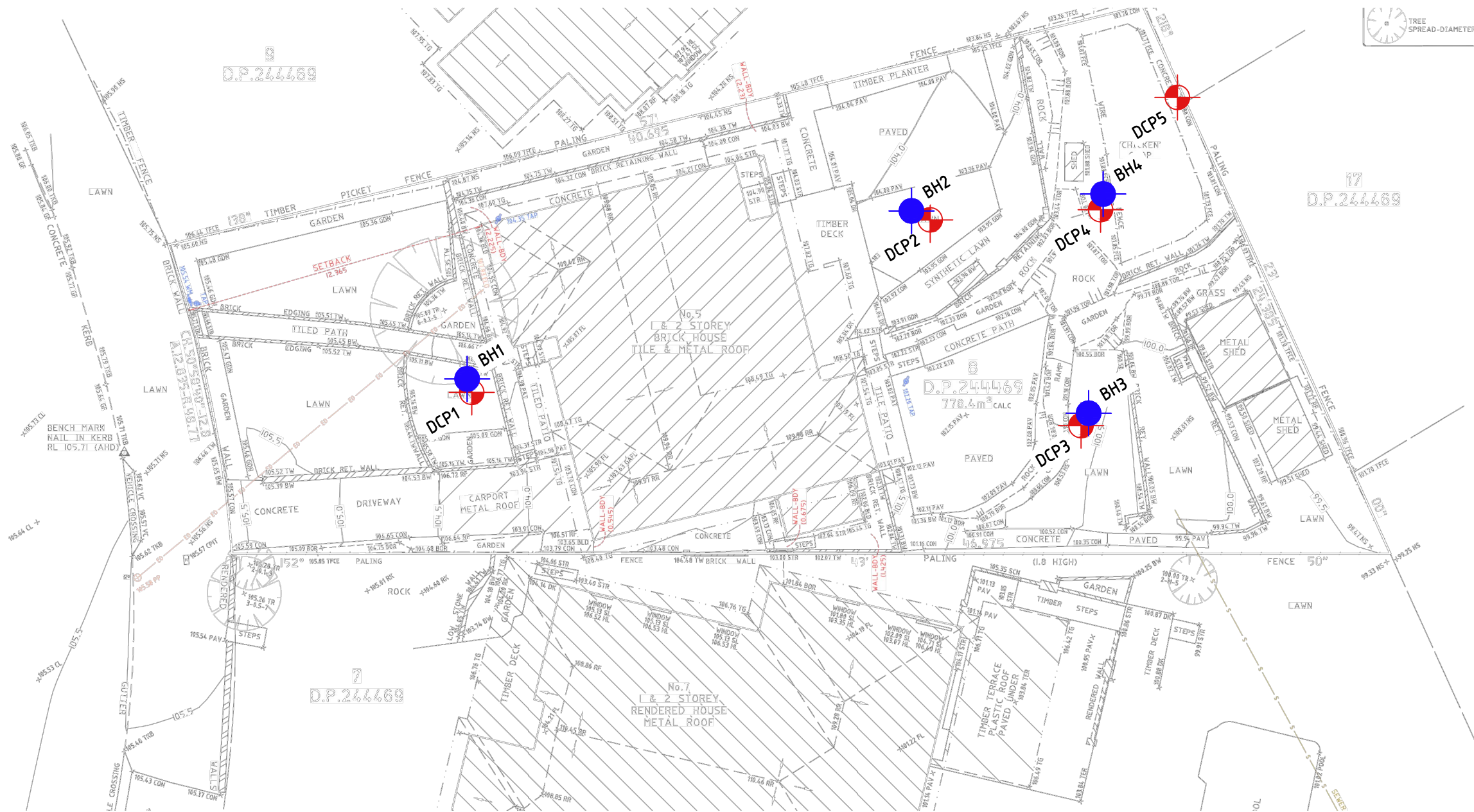
SITE PLAN/GROUND TEST LOCATIONS SCALE NTS
