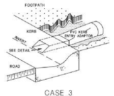
ROLLED KERB AND "ANGLE CUT" KERB
