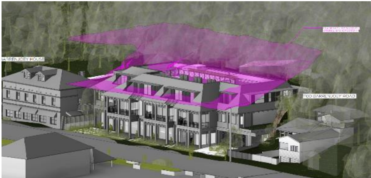
Figure 2 – Interpolated undisturbed building height blanket diagram showing the location and extent of building elements located above the 8.5 metre building height standard.
