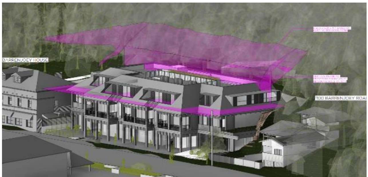
Figure 1 – Building height blanket diagram showing the location and extent of building elements located above the 8.5 metre building height standard calculated in accordance with Merman
