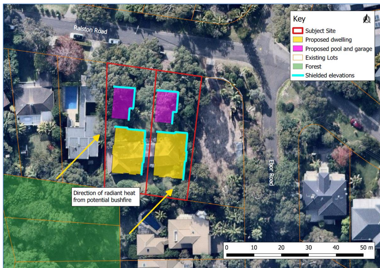
Figure 7. Shielding Diagram. Source: NearMap (2019) with overlays by BFCS P/L: Aerial Photography Date: 02/07/2019
