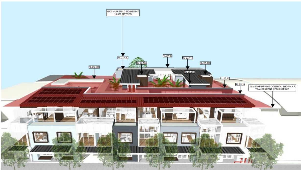
Figure 7 – Building height blanket diagram showing non-compliant building height elements
