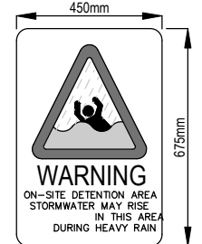
ON-SITE DETENTION WARNING SIGN NTS
