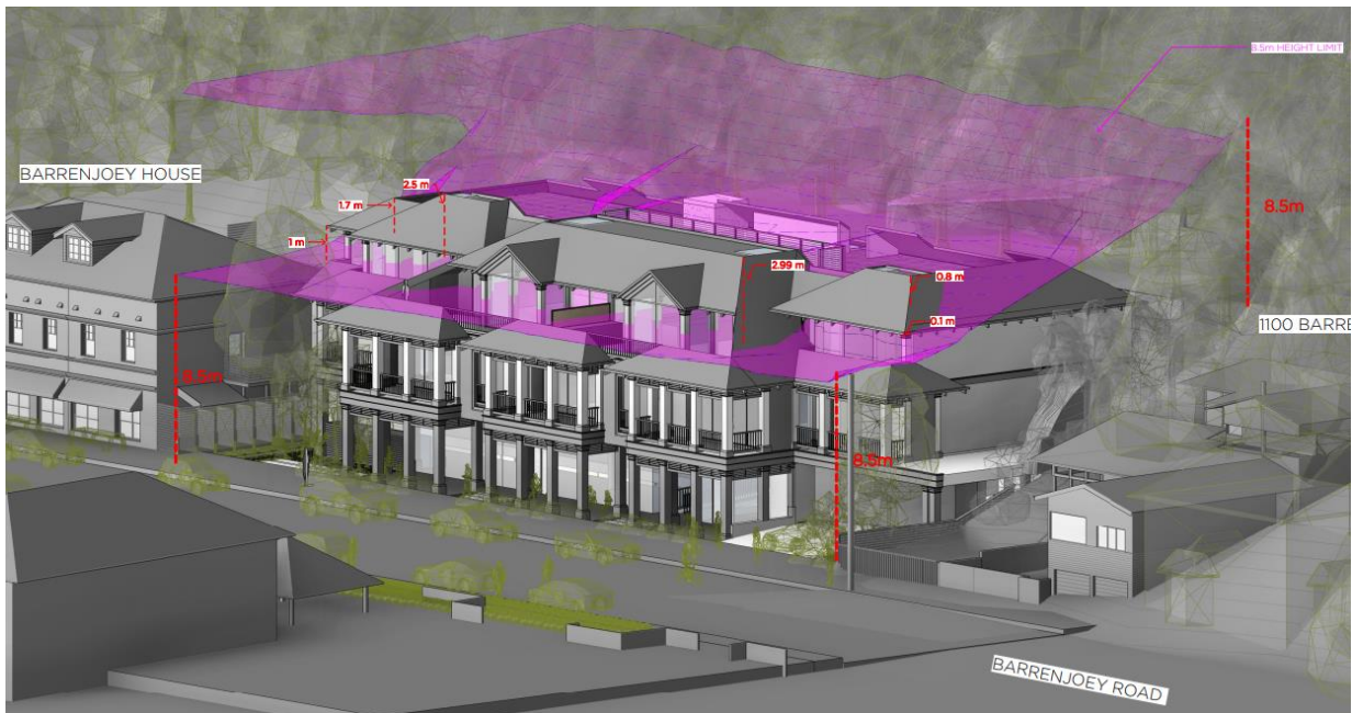
Figure 6 – Building height diagram showing non-compliant building height elements projecting through the 8.5 metre height blanket.
