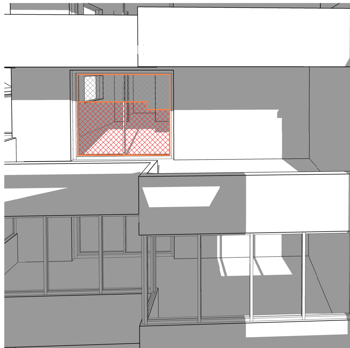
1c LEVEL 2 - APPROVED DA 10AM - % AREA OF GLAZING WITH DIRECT SUNLIGHT = 4.25m 2 (63.1%)
