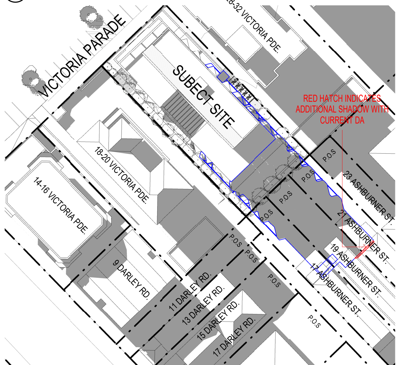
7c DA13 1:500 SOLAR ACCESS PLAN - CURRENT DA - 3PM
