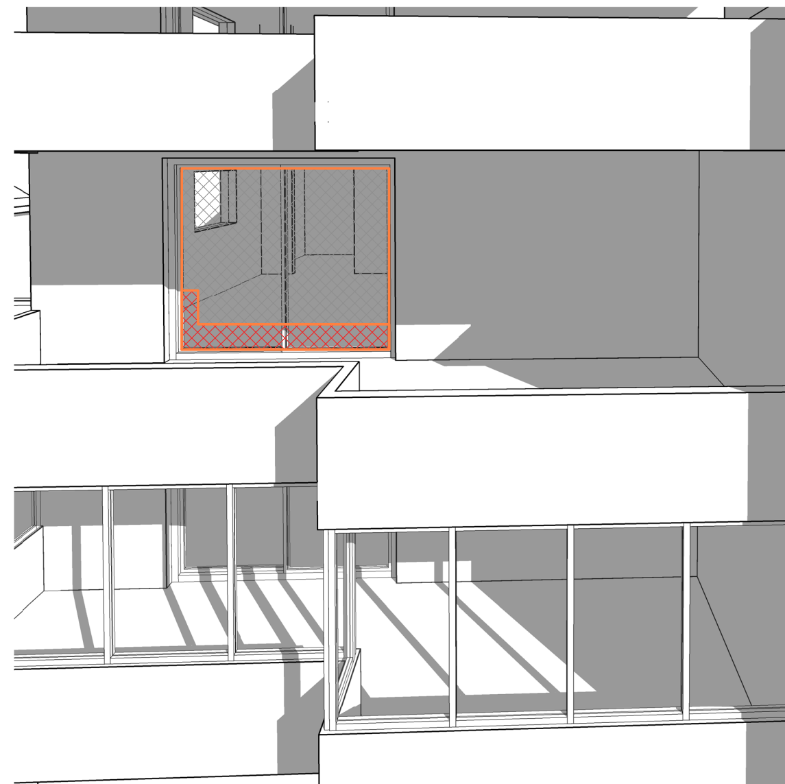
6c LEVEL 2 - PROPOSED DA 12PM - % AREA OF GLAZING WITH DIRECT SUNLIGHT = 1.05m 2 (15.60%)
