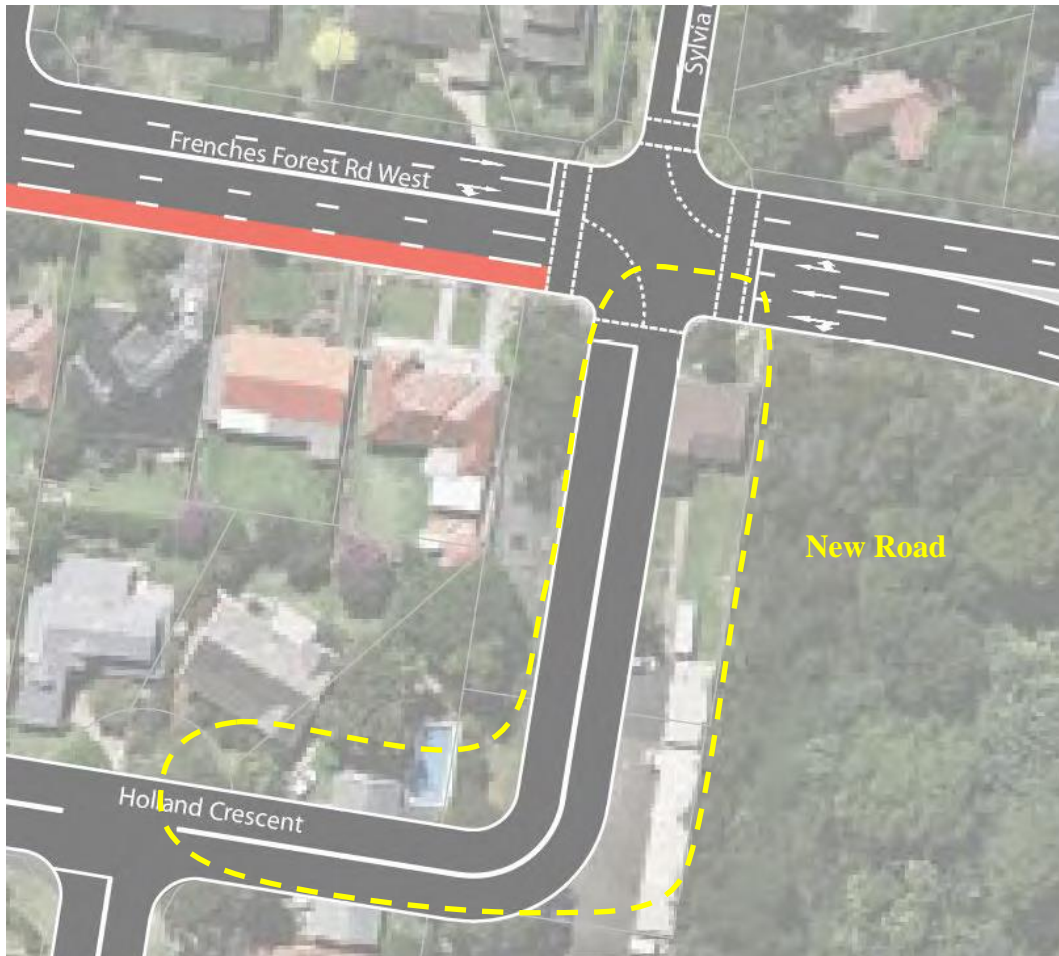
Figure 20: New Road from Holland Crescent to Frenchs Forest Road West
