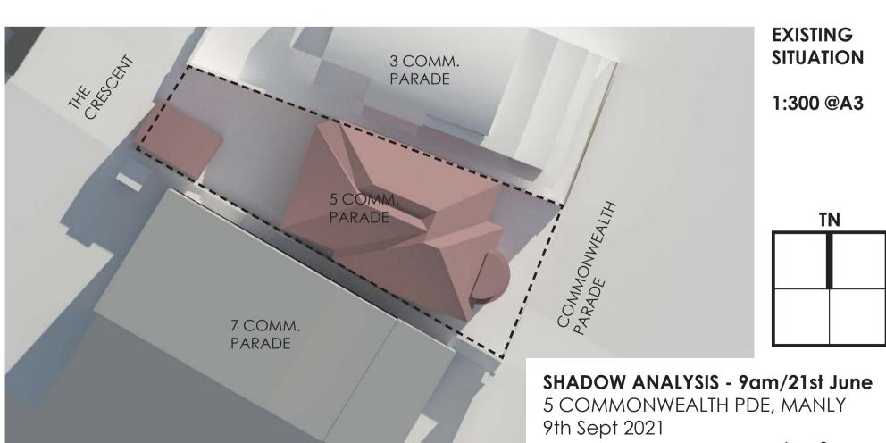
NOTE: ALL 3D MODELS HAVE BEEN ACCURATELY MODELLED AS PER EXISTING SURVEY DATA, APPROVED ARCHITECTURAL PLANS AND PROPOSED ARCHITECTURAL PLANS. SHADOWS SHOWN AS CAST ON THE 21st JUNE.
