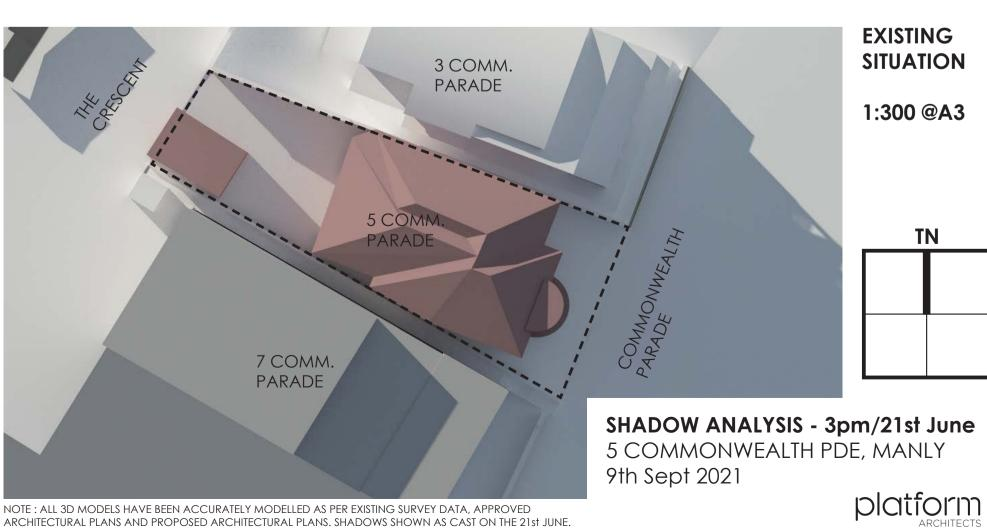
NOTE: ALL 3D MODELS HAVE BEEN ACCURATELY MODELLED AS PER EXISTING SURVEY DATA, APPROVED ARCHITECTURAL PLANS AND PROPOSED ARCHITECTURAL PLANS. SHADOWS SHOWN AS CAST ON THE 21st JUNE.
