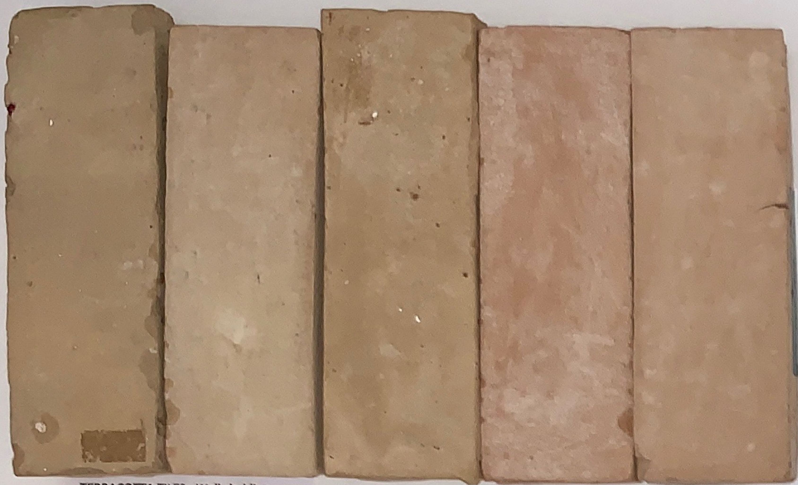
TERRACOTTA TILES - Wall cladding
