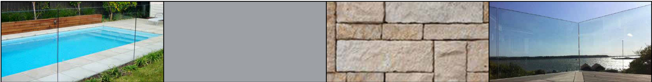
FE. BALUSTRADE EXTERNAL / POOL FENCE GLASS PANELS SET INTO SLAB CLEAR GLASS RF. ROOF METAL SHEET ROOFING COLORBOND WINDSPRAY OR SIMILAR ST. STONE CLAD RANDOM STONE TUSCAN LIMESTONE GB. GLASS BALUSTRADE FRAMELESS CLEAR GLASS
