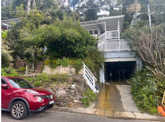
Photo 1: Site frontage, note significant seepage from the rear wall of the garage
