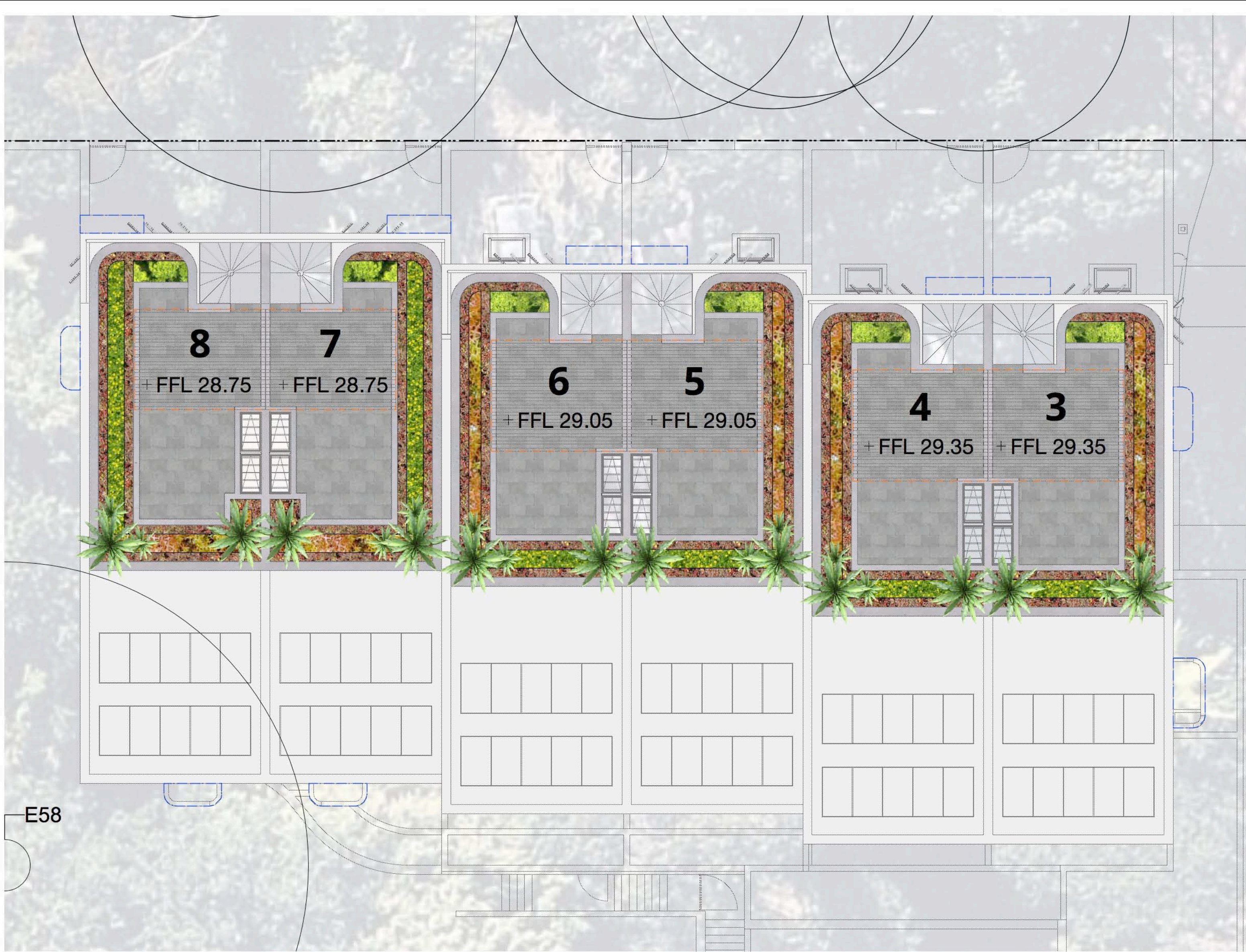
02 Rooftop Terrace Detailed Plan @ 1:100
