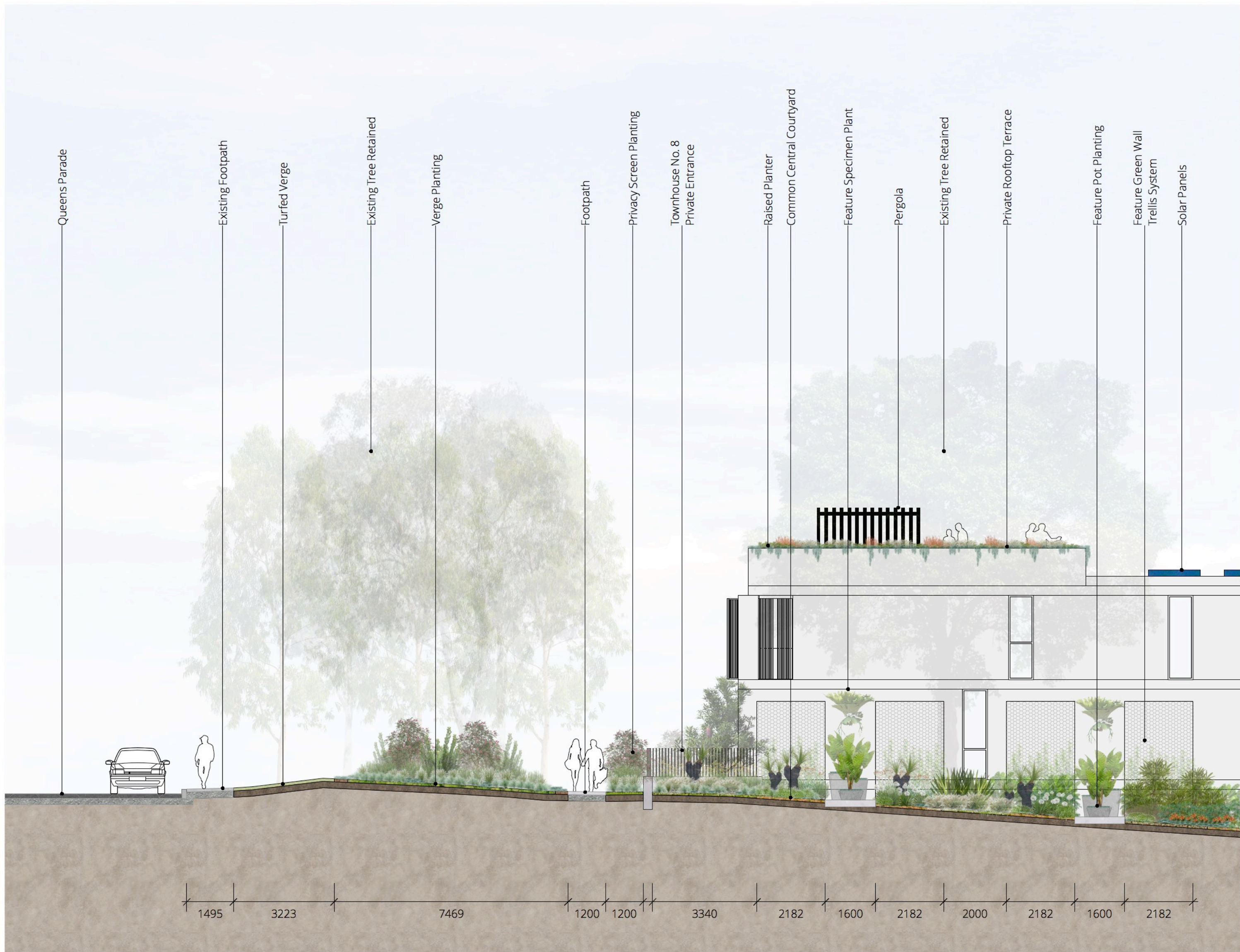
01 Queens Parade and Central Courtyard Sectional Elevation @ 1:100
