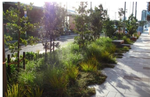
Figure 10: Bioswales could be located in streetscapes to improve the water quality in the precinct
