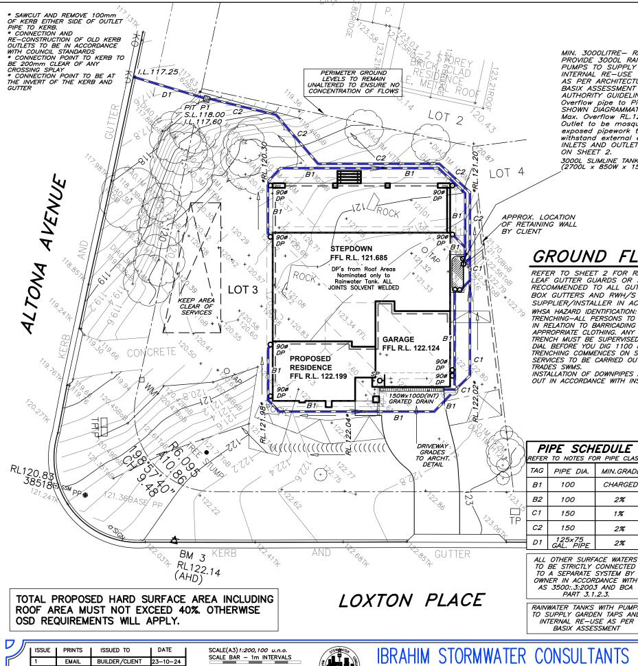
MIN. 3000LITRE— RAINWATER TANK PROVIDE 3000L RAINWATER TANK WITH PUMPS TO SUPPLY GARDEN TAPS AND INTERNAL RE-USE TO BE CONNECTED AS PER ARCHITECTURAL DETAILS, BASIX ASSESSMENT AND WATER AUTHORITY GUIDELINES. Overflow pipe to Pit P1. LOCATION SHOWN DIAGRAMMATIC ONLY. Max. Overflow RL.123.08m Outlet to be mosquito proofed. All exposed pipework to be painted to withstand external elements.PIPE INLETS AND OUTLETS AS PER DETAILS ON SHEET 2.
