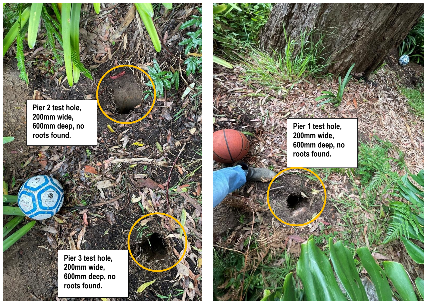
Figure 6: Preliminary root investigation holes, hand excavated, in locations of proposed piers 1,2 and 3, within SRZ of Tree 3. No significant structural roots were found. Other proposed pier locations were not investigated due to presence of existing concrete driveway.
