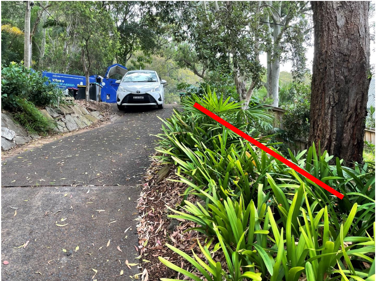
Figure 3: The driveway and carport must be elevated above the old driveway. The driveway and carport are wider than the existing driveway (roughly along the red line). Existing gradients must be retained under the driveway so that roots are minimally damaged. The new driveway must have a gap between the driveway and the existing sloping wall on the boundary, so that water can pass under the new driveway to water the roots. The old driveway concrete will be removed prior to construction of the new elevated driveway, but it should be left in place until work on the house has been completed.
