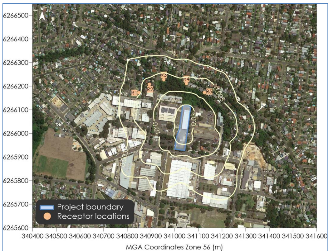
Figure B-10: Predicted incremental 1-hour average benzene concentrations ( \mu\text{g}/\text{m}^3 )
