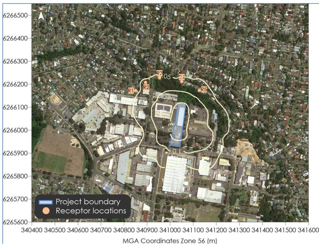
Figure B-11: Predicted incremental 1-hour average formaldehyde concentrations ( \mu\text{g}/\text{m}^3 )
