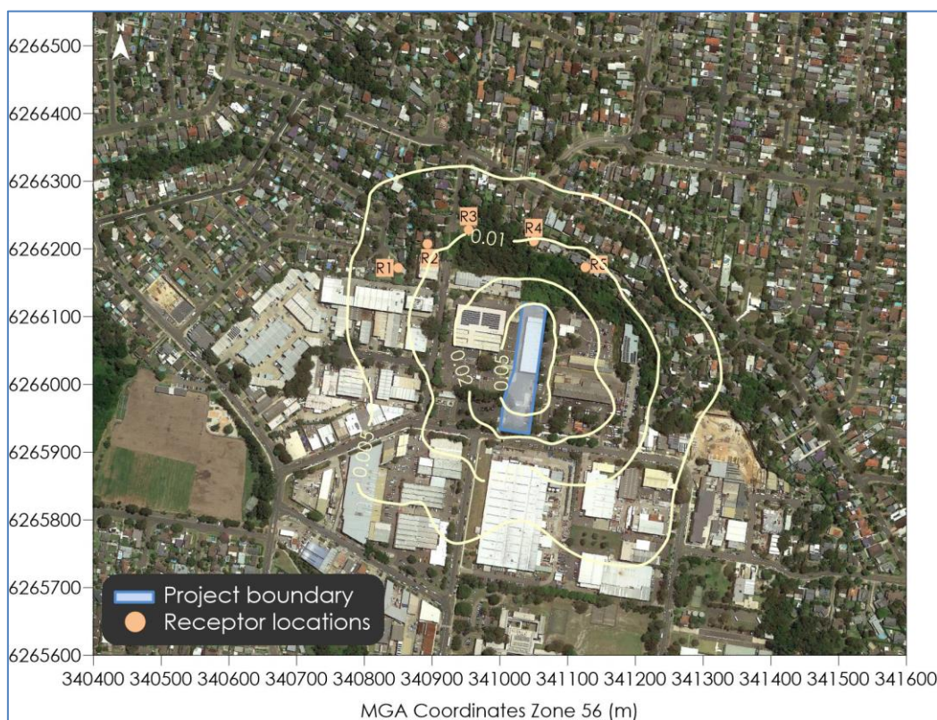
Figure B-12: Predicted incremental 1-hour average PAH concentrations ( \mu\text{g}/\text{m}^3 )
