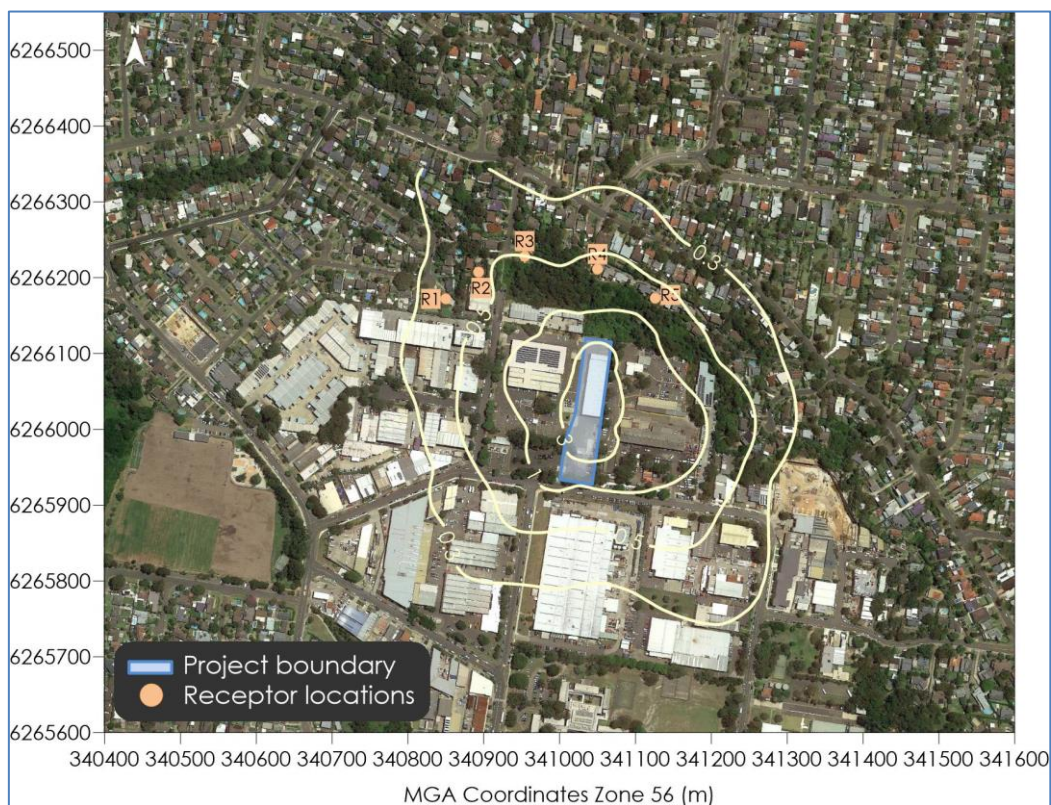
Figure B-9: Predicted incremental 8-hour average CO concentrations ( \mu\text{g}/\text{m}^3 )
