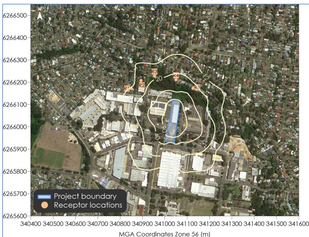
Figure B-6: Predicted incremental 1-hour average \text{NO}_2 concentrations ( \mu\text{g}/\text{m}^3 )
