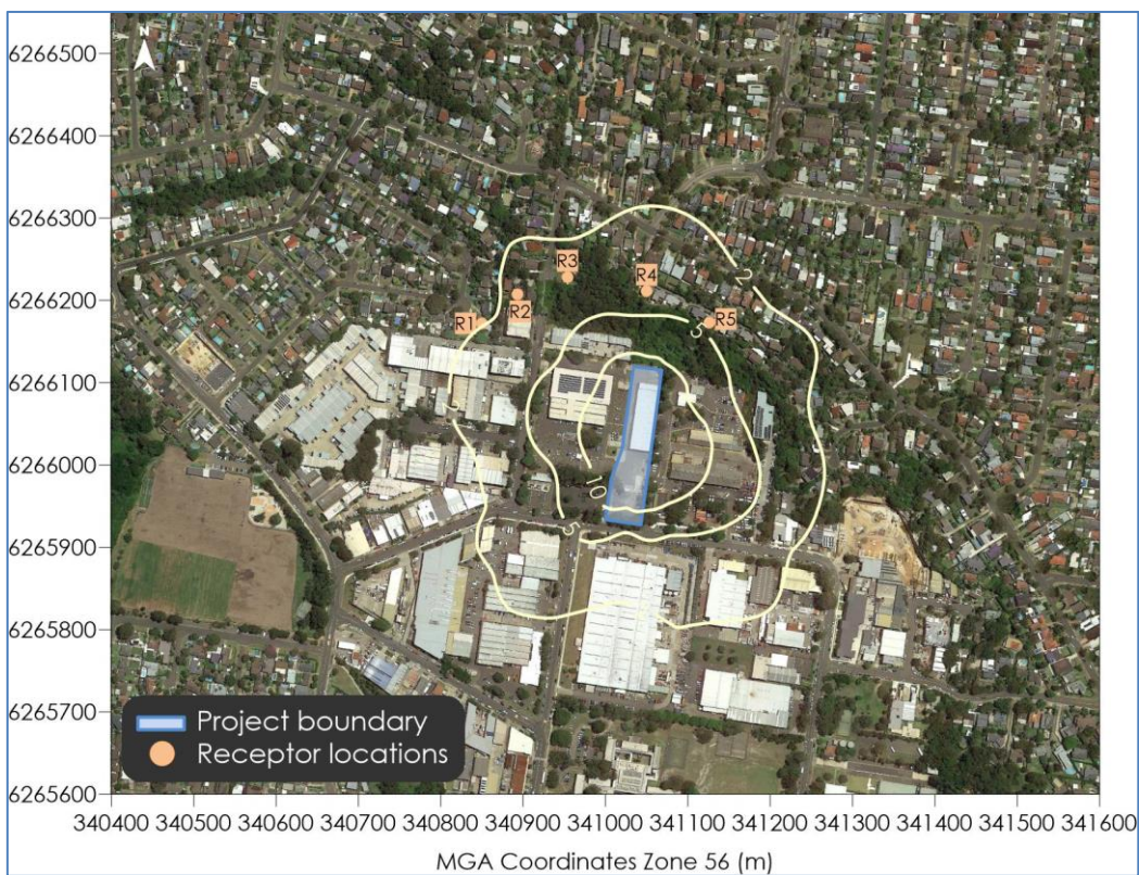
Figure B-8: Predicted incremental 1-hour average CO concentrations (µg/m 3 )
