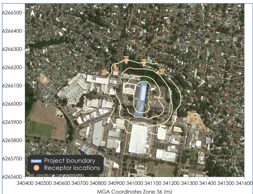
Figure B-14: Predicted incremental 1-hour average xylene concentrations ( \mu\text{g}/\text{m}^3 )
