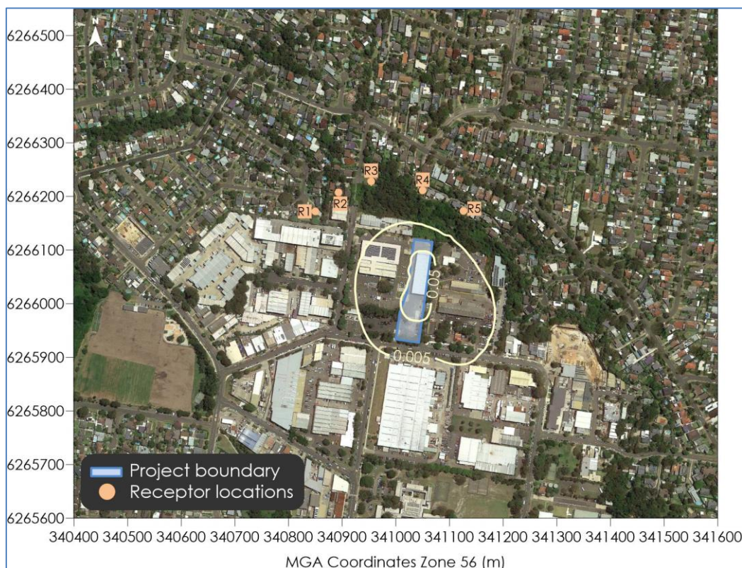
Figure B-5: Predicted incremental annual average TSP concentrations ( \mu\text{g}/\text{m}^3 )
