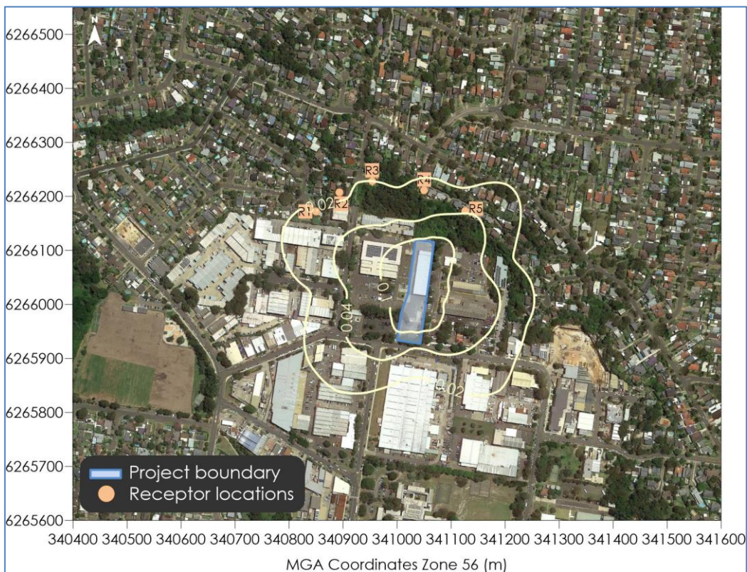
Figure B-3: Predicted incremental 24-hour average PM 10 concentrations (µg/m 3 )
