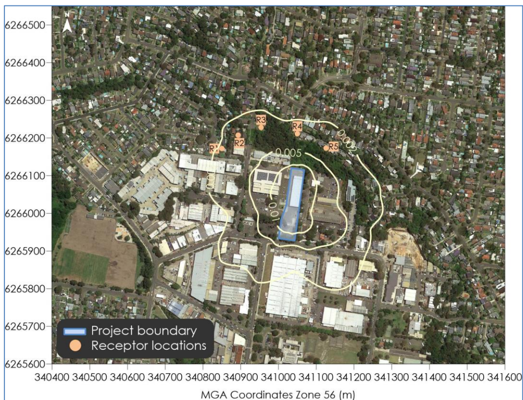
Figure B-13: Predicted incremental 1-hour average toluene concentrations ( \mu\text{g}/\text{m}^3 )
