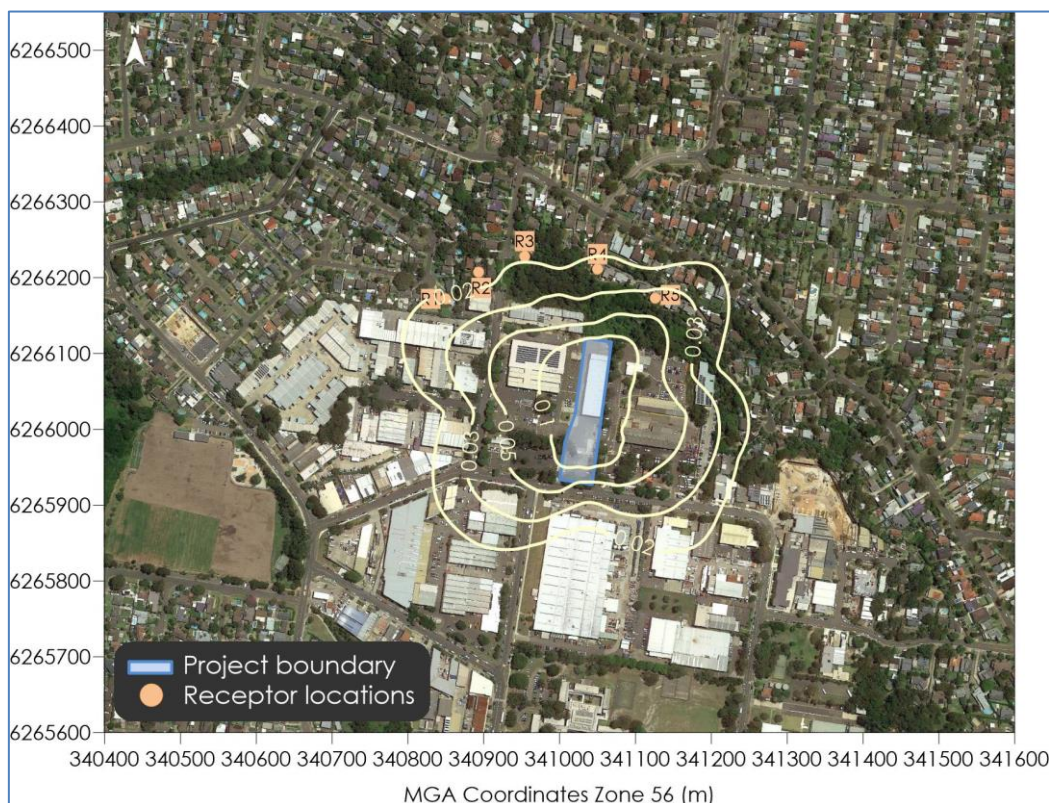
Figure B-1: Predicted incremental 24-hour average PM 2.5 concentrations (µg/m 3 )
