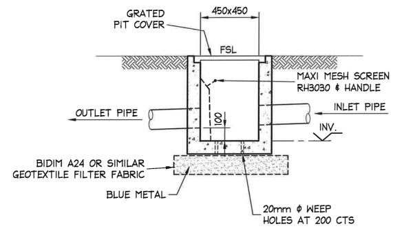
PRECAST OR CAST INSITU PIT REFER STORMWATER NOTES ALTERNATE POLYPROPYLENE PIT BY MANUFACTURER
