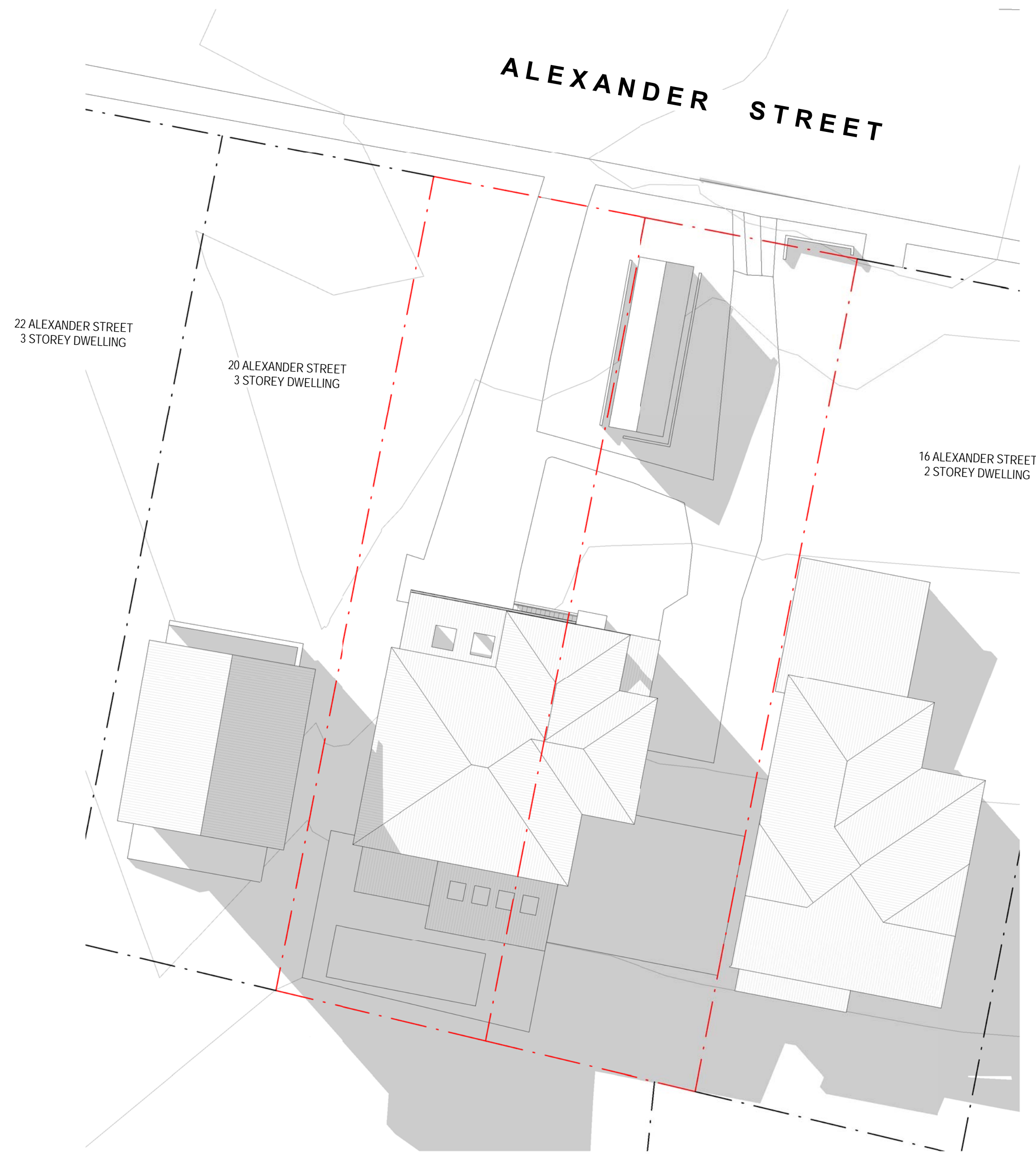
1 EXISTING SHADOW DIAGRAM - 3PM JUNE 21ST DA503 / 1 : 200 @ A1
