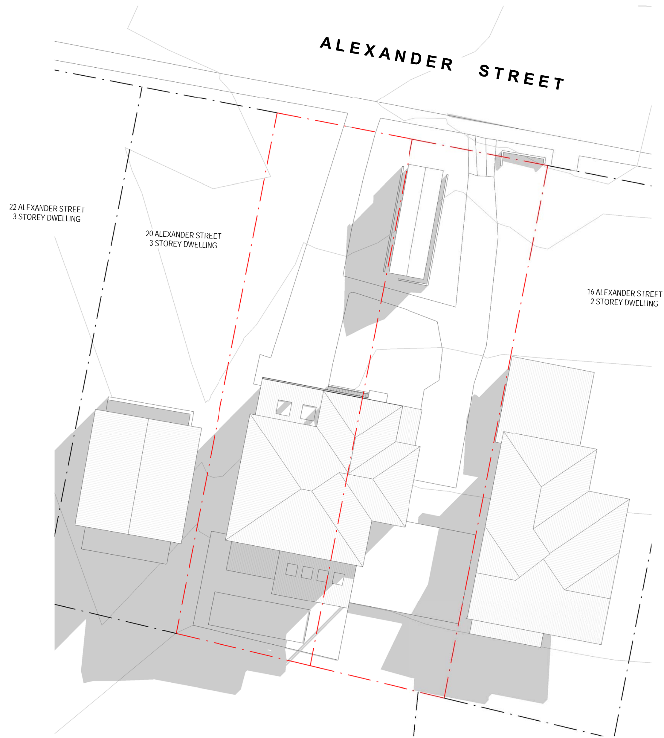
1 EXISTING SHADOW DIAGRAM - 9AM JUNE 21ST DA500/ 1:200 @ A1
