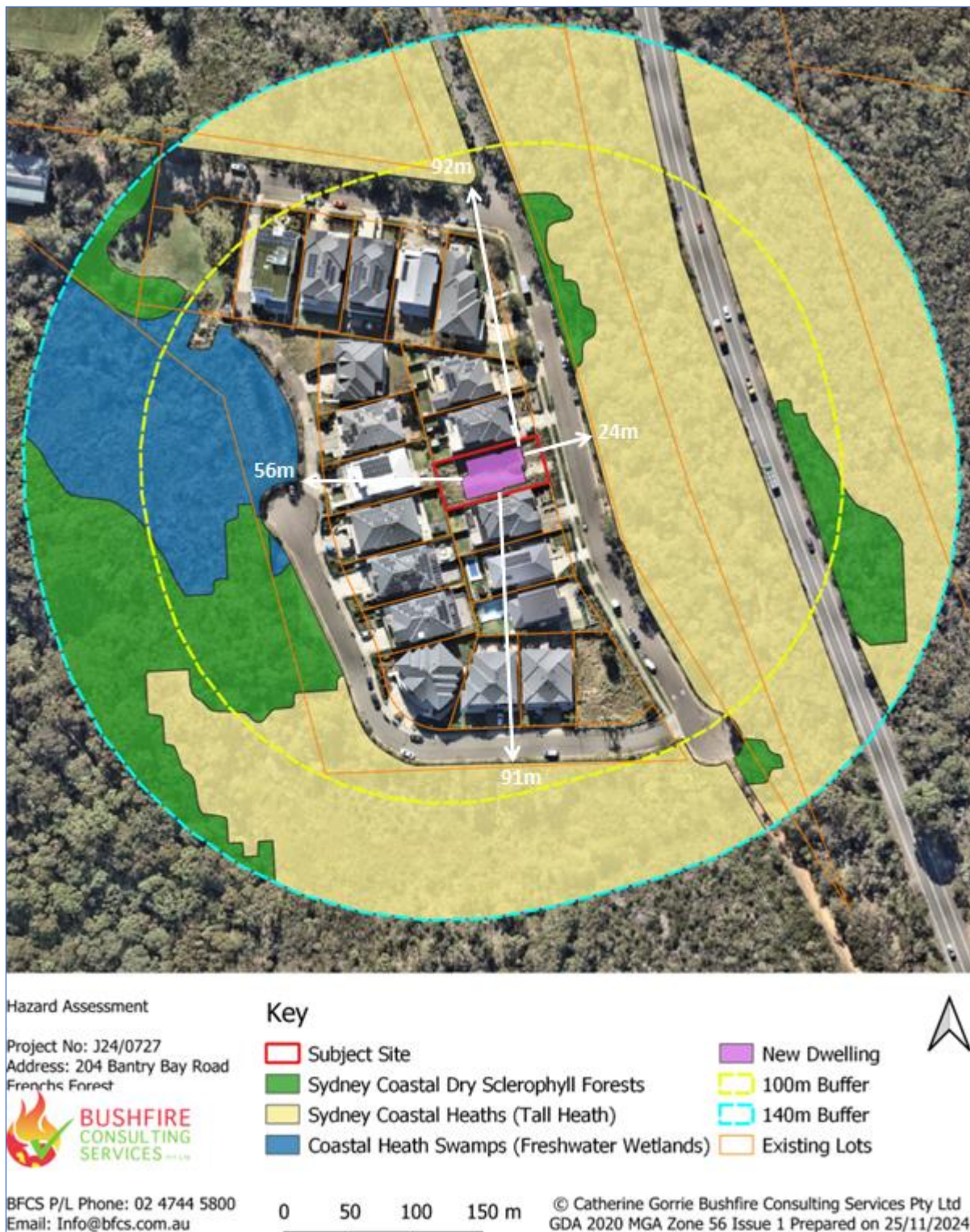
Figure 5. Hazardous vegetation affecting the subject building. Source: NearMap (2024) with overlays by BFCs P/L. Aerial Photography date: 30/10/2024
