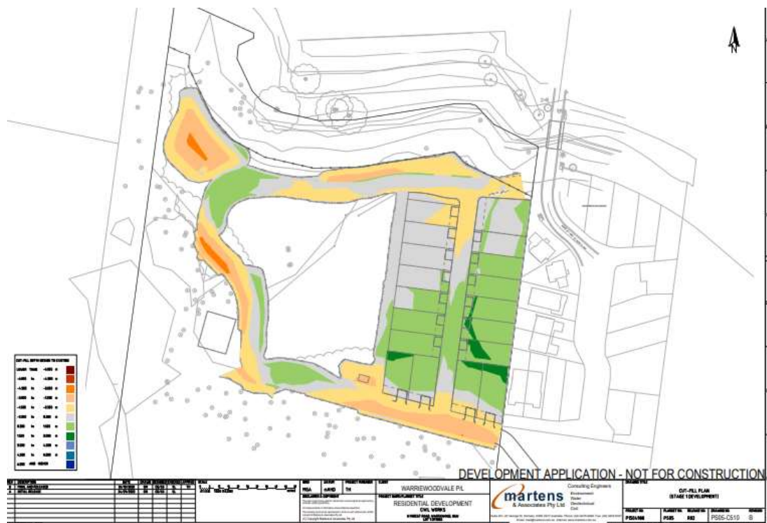
Figure 2 – Site plan showing cut and fill. The light green shows 1.5m fill.
