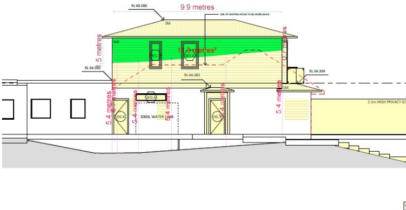
Image 2: southern elevation envelope non-compliance
