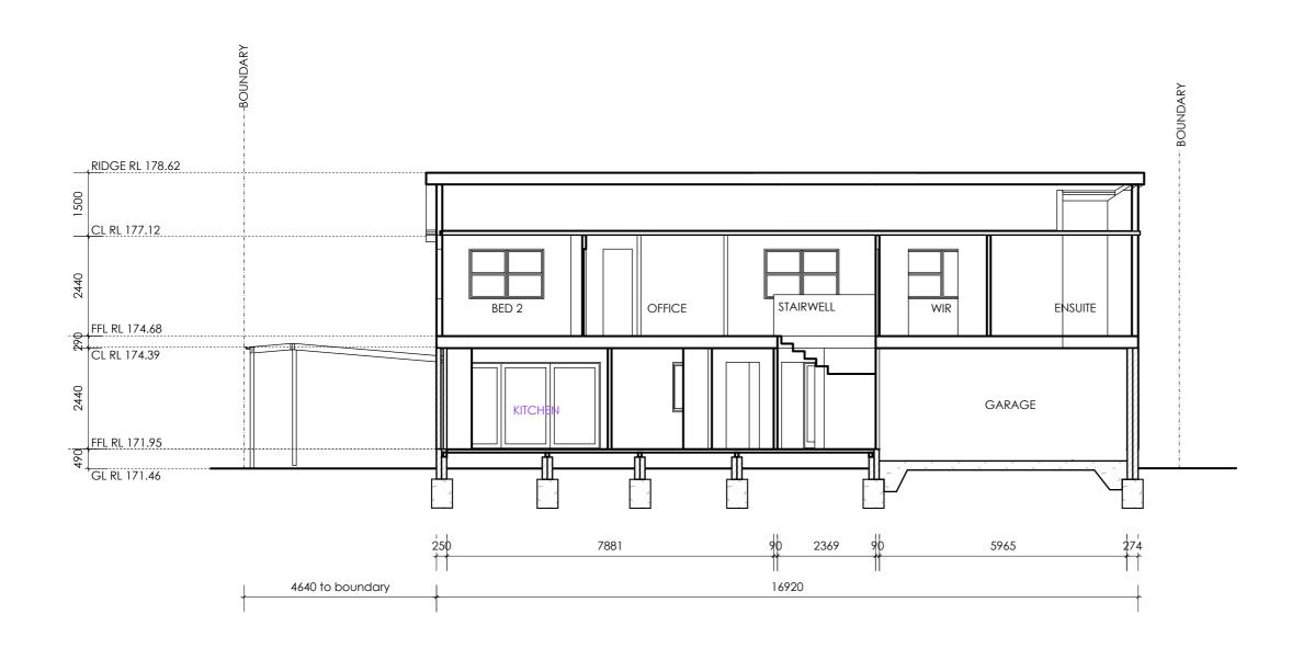
90 BY 45 H2 STUDS @ 600c 90 BY 45 H2 NOGGINS @ 1.200c MAX 90 BY 45 H2 PLATES/ 2 TOP 1 BOTTOM **EXTERIOR WALLS CLAD IN Weathertex** Eaves 4.5mm fibro, H mold
