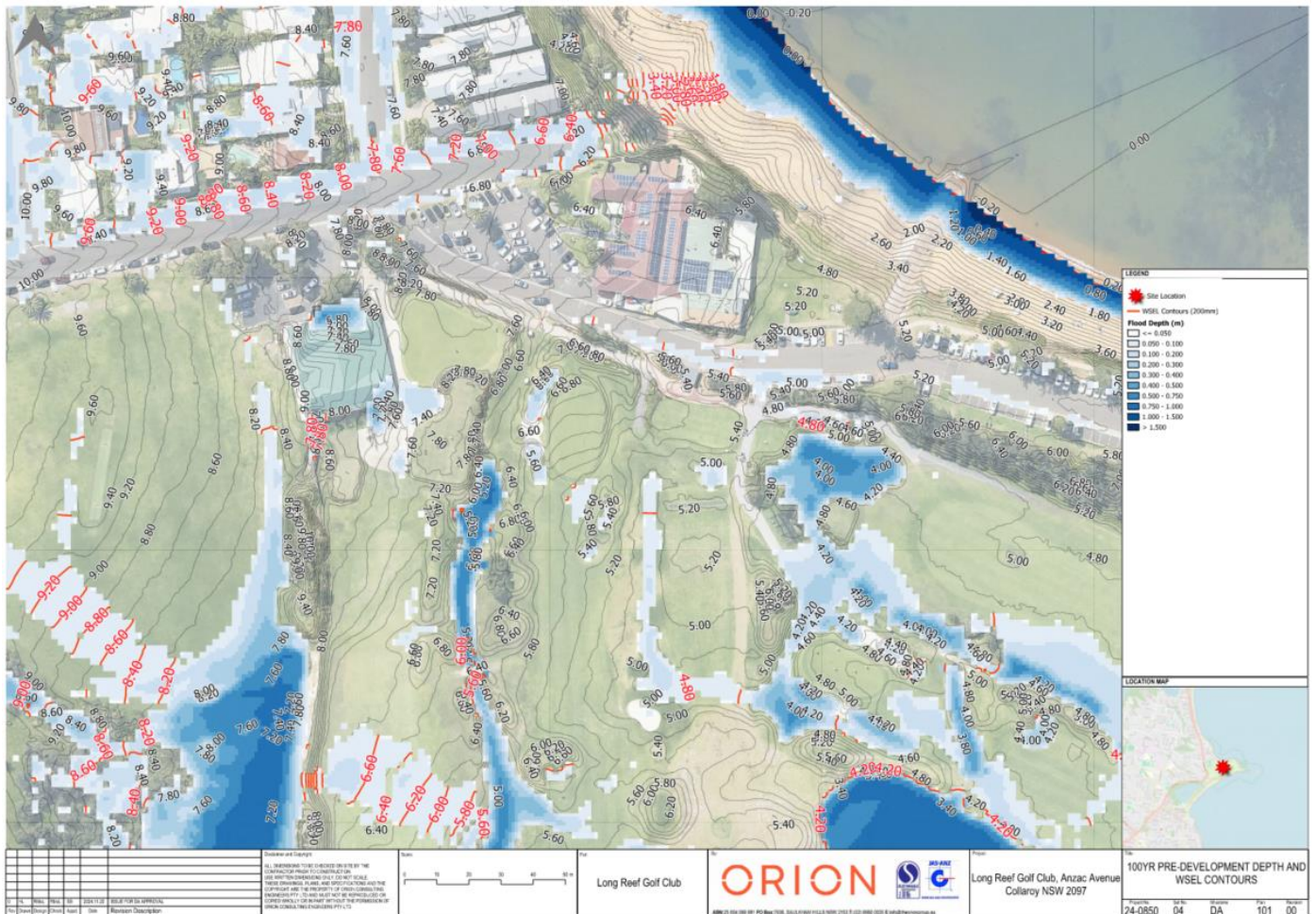
Figure 12 Existing 1% AEP flood depth – project vicinity
