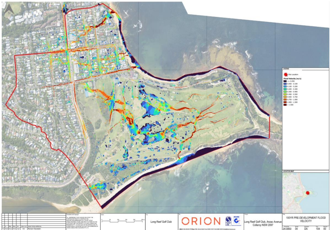
Figure 15 1% AEP flood velocity in the catchment area
