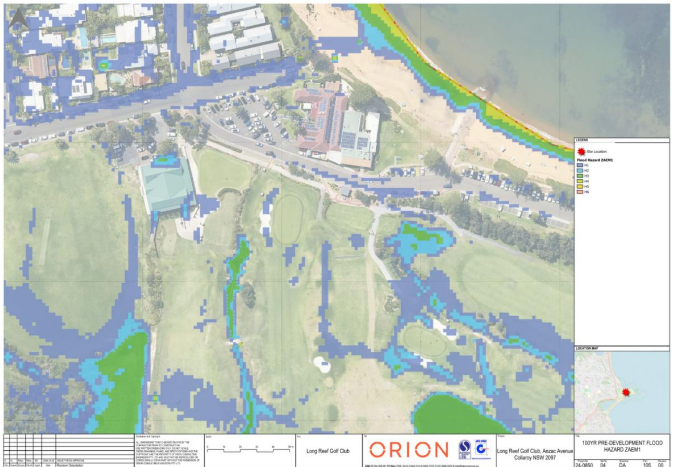
Figure 16 flood hazard near the Golf Club H1 flood hazard is noted as safe for people, vehicles and building
