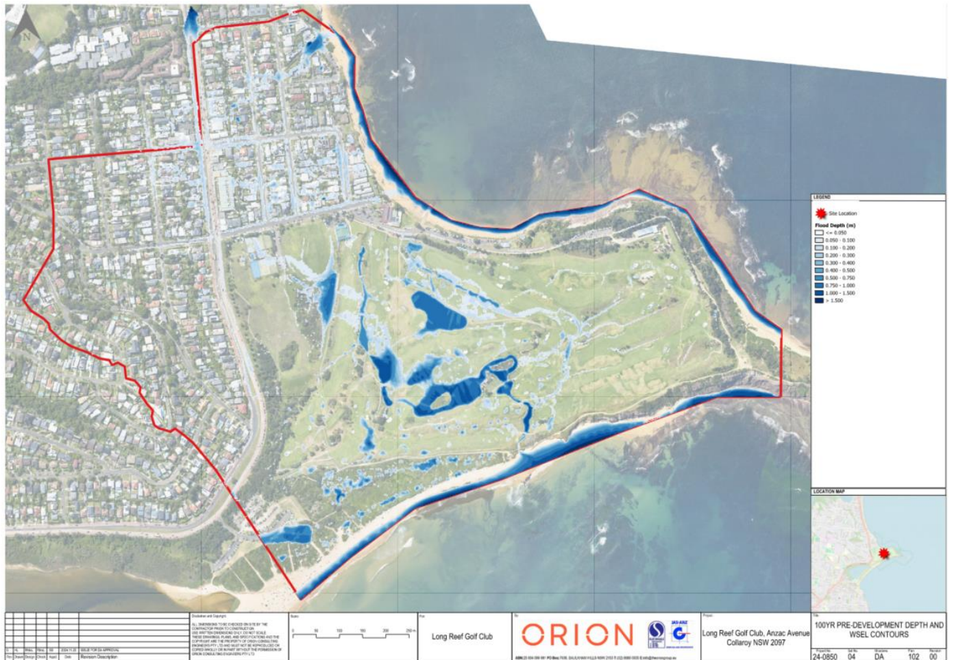
Figure 13 Existing 1% AEP flood depth – catchment view
