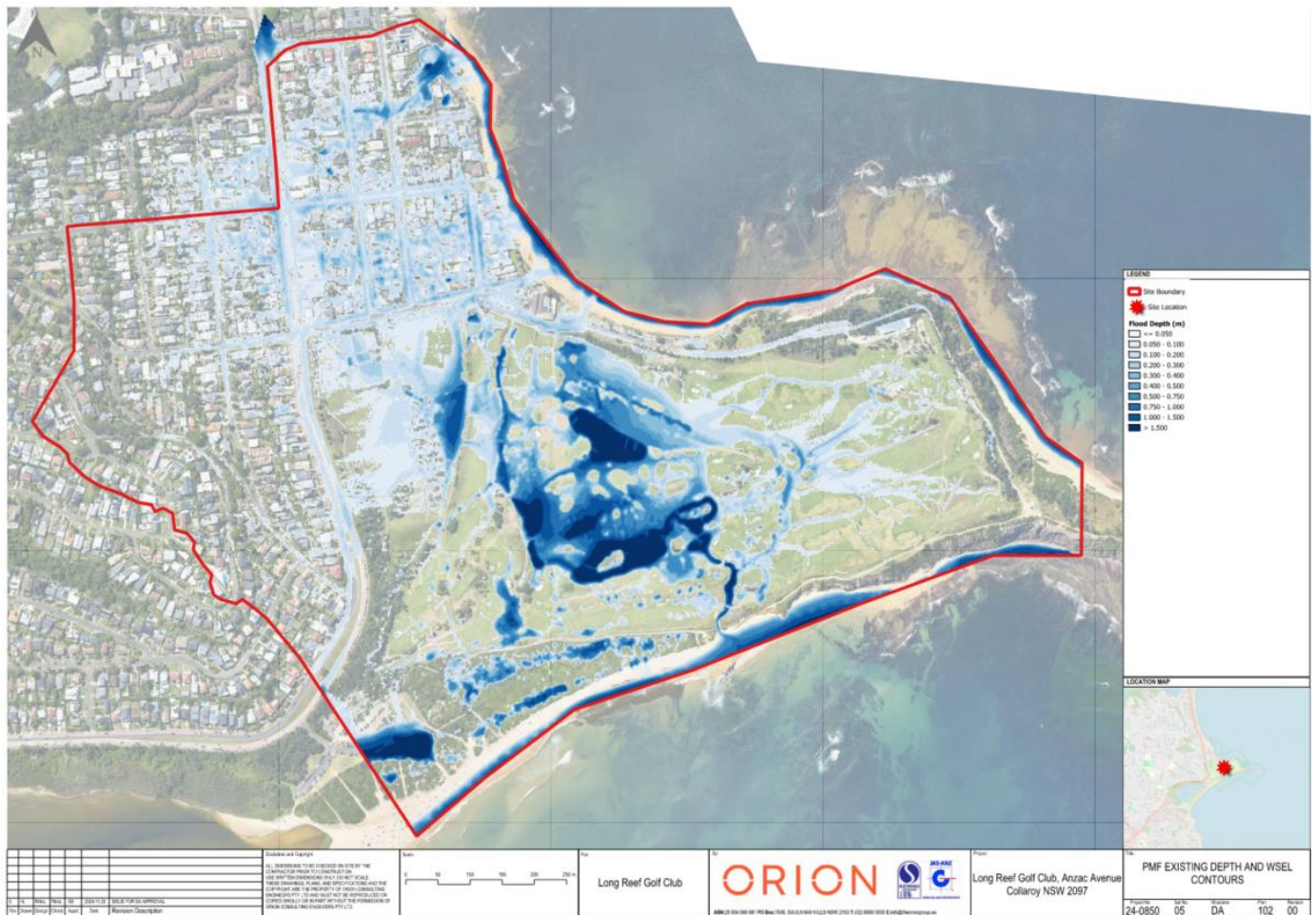
Figure 20 PMF flood levels in the catchment
