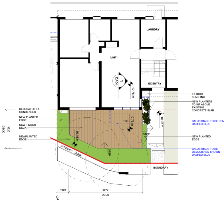
Figure 1 : Ground Floor level
