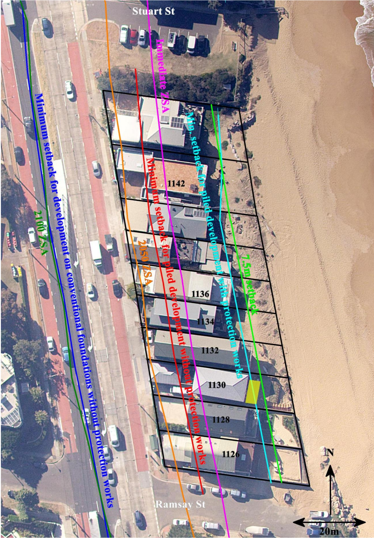
Figure 4: Coastline hazard lines at subject property, with footprint of proposed balcony in yellow (aerial photograph taken 17 August 2018)
