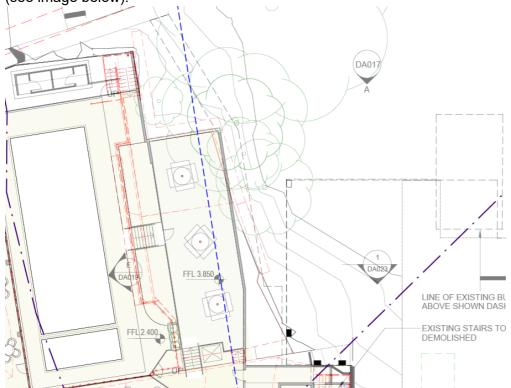
Any new retaining structures shall be wholly contained within the existing footprint of the upper pool terrace area, so as not to disturb existing trees 1, 2, and 4. The proposed service and fire egress pathway is labelled 'indicative location' on the plans. This pathway shall be located and designed in collaboration with the Arborist to ensure trees 1, 2, and 4 can be retained. The Arborist shall provide updated commentary on any design changes and to confirm the retention of trees 2 and 4.
