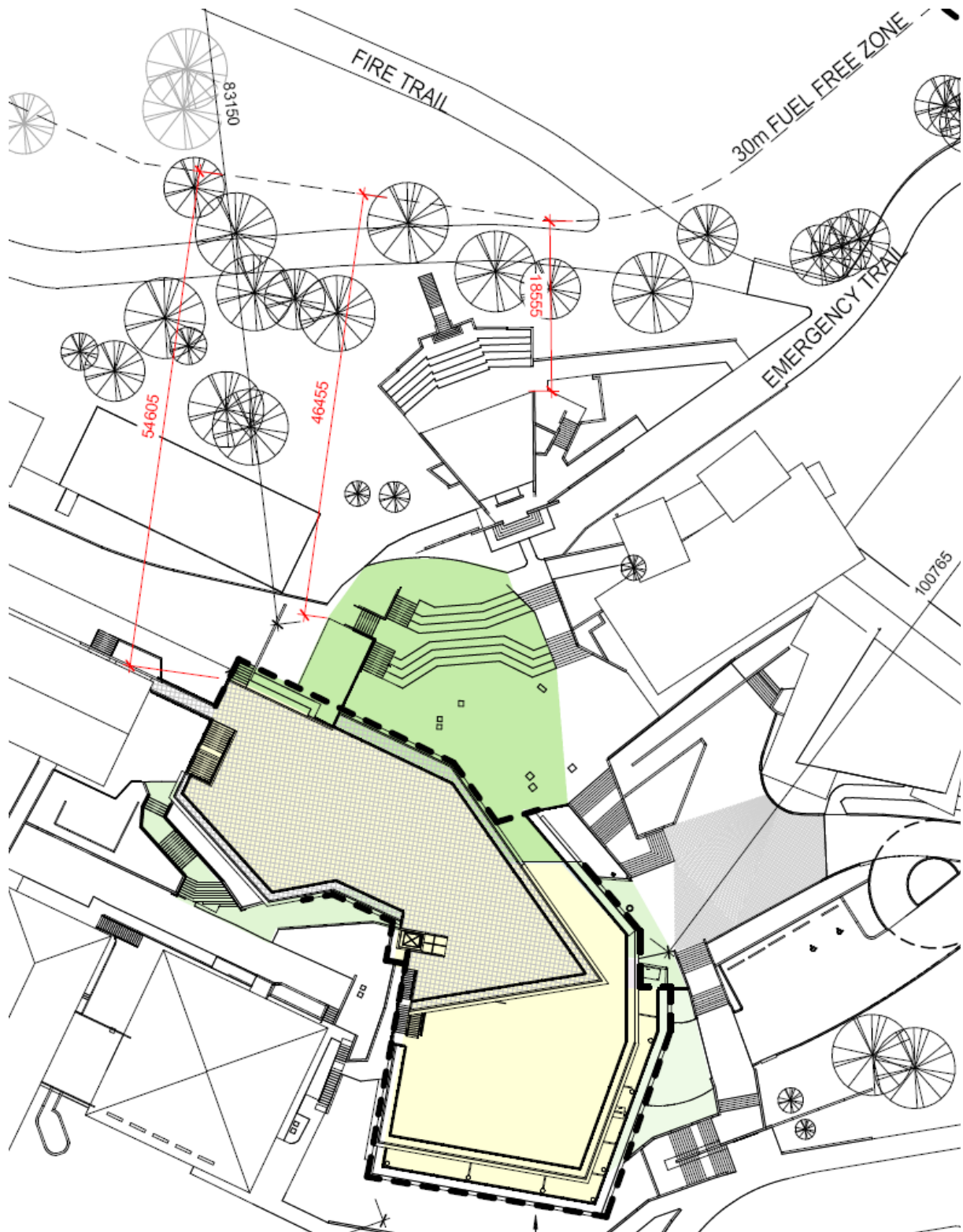
Figure 12 - Site Plan showing the available setbacks to the outer edge of the approved and maintained Asset Protection Zone.
