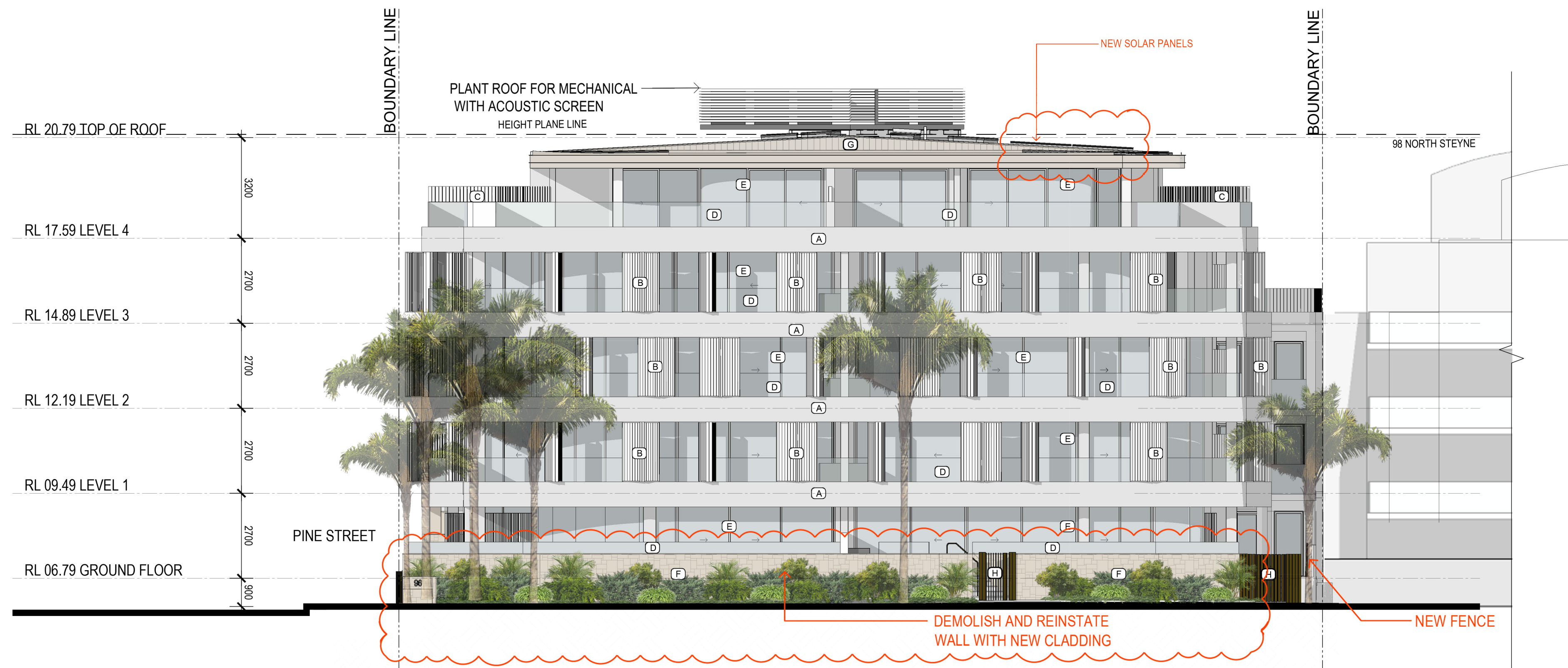
PROPOSED EAST ELEVATION (NORTH STEYNE) scale - 1:100@A1
