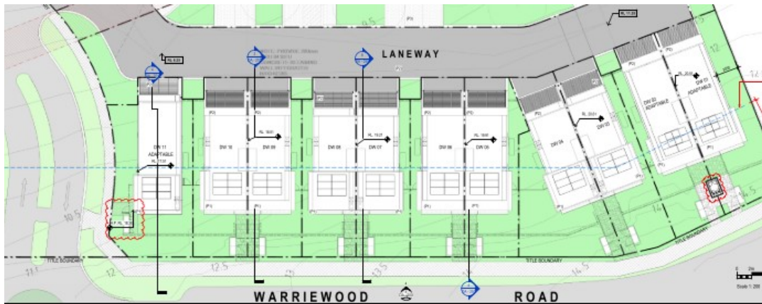
Plan showing the location of the platform lift to dwelling 1 and 2 and the change to the entry to dwelling 11.
