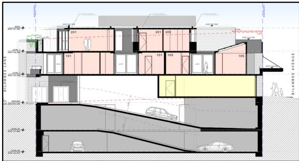
Figure 2: Extract of Section AA plan showing LEP 8.5m height line (Source: Benson McCormack Architecture, Project No. 2012A)
