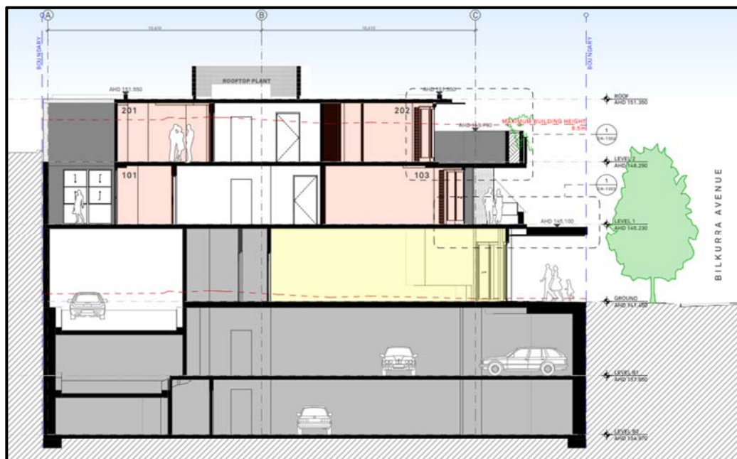
Figure 3: Extract of Section BB plan showing LEP 8.5m height line (Source: Benson McCormack Architecture, Project No. 2012A)
