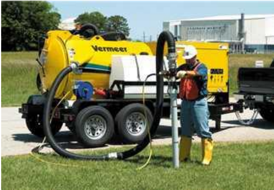
Figure 17 – Aero/Hydro vacuum excavator
