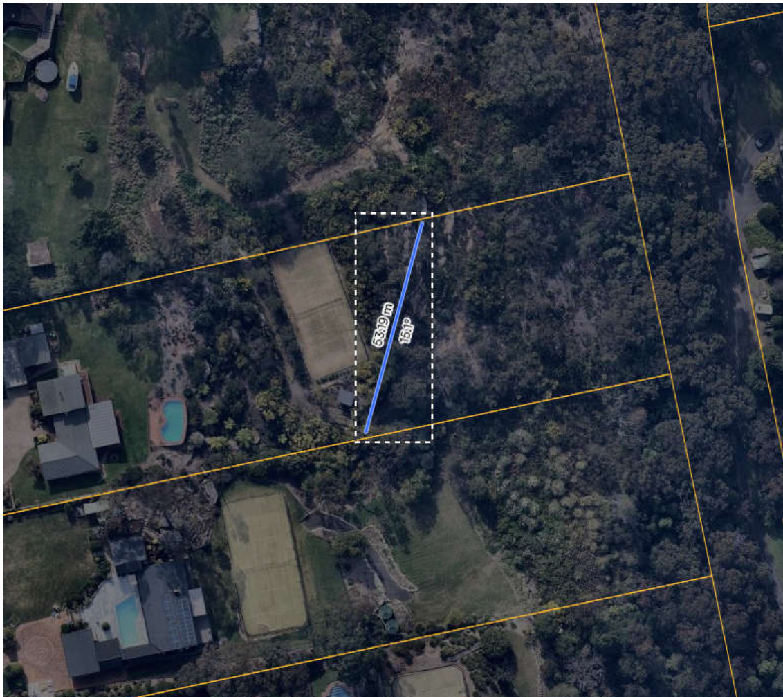
Figure 2.3 – Effective width of flame used for calculation although 60m was used in the calculation - see Figure 2.4 below
