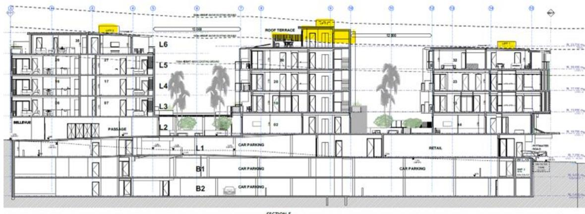
**Figure 1** – Section F with the 16.9m building height line plotted and non-complying elements highlighted yellow (Source: Gartner Trovato)
