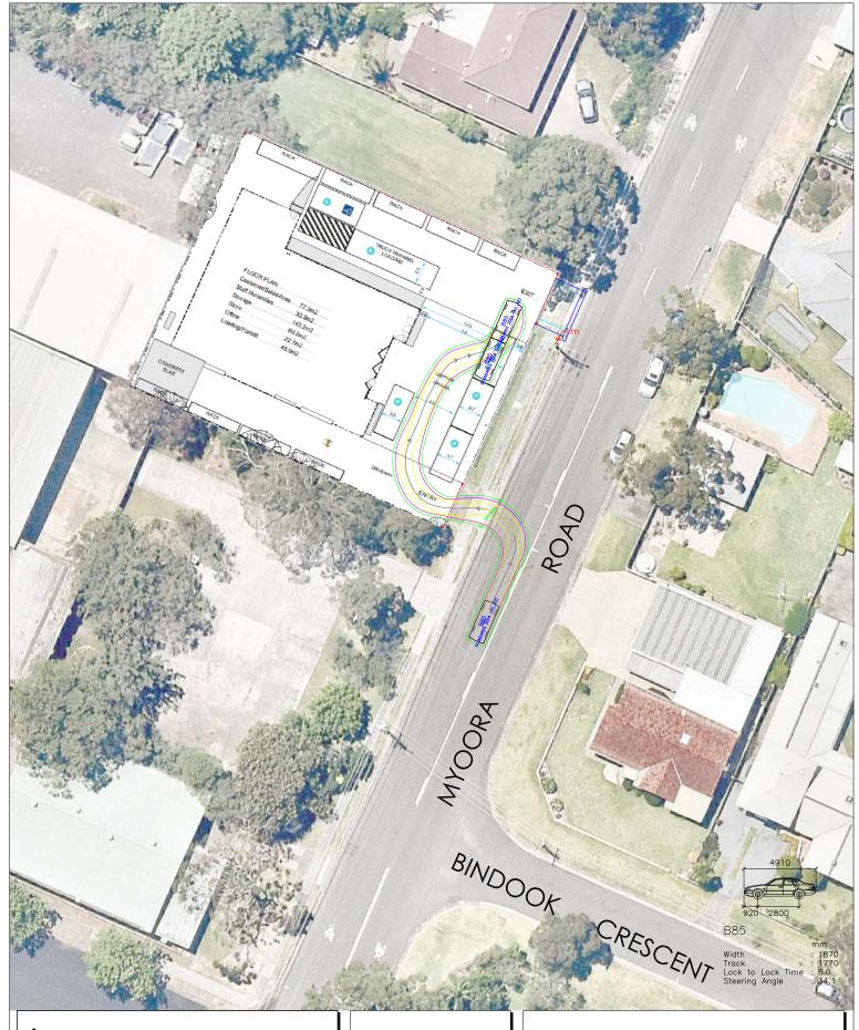
This drawing has been prepared using vehicle modelling computer software AutoTURN PRO10 in conjunction with AutoCAD 2018. The vehicle used is based upon vehicle data provided by Austroads and incorporates a reasonable degree of tolerance. However, it is not possible to account for all vehicle types/characteristics and/or driver ability.
