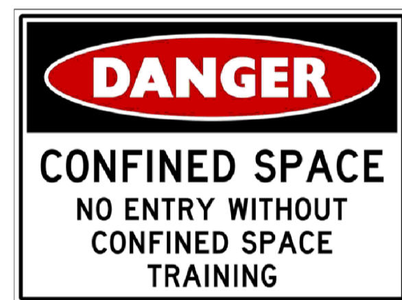
DETAIL - CONFINED SPACE SIGN TO BE PLACED INSIDE OSD TANK & BASEMENT PUMPOUT PIT NTS
