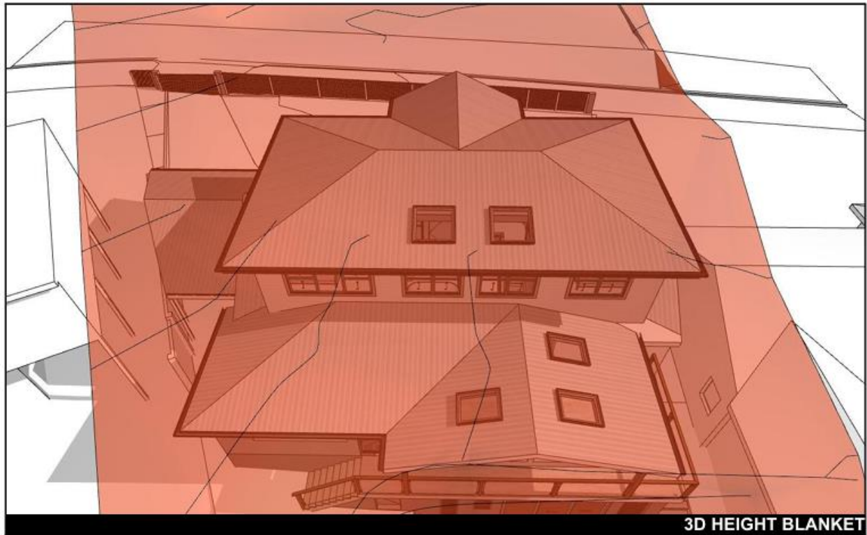
Figure 2. 3D Height Blanket prepared by Action Plans illustrating compliance with the maximum height control using the Bettar calculation method
